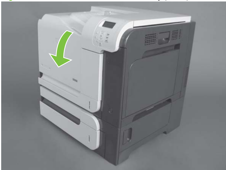
Figure 6-44 Remove the front-door assembly (1 of 2)
