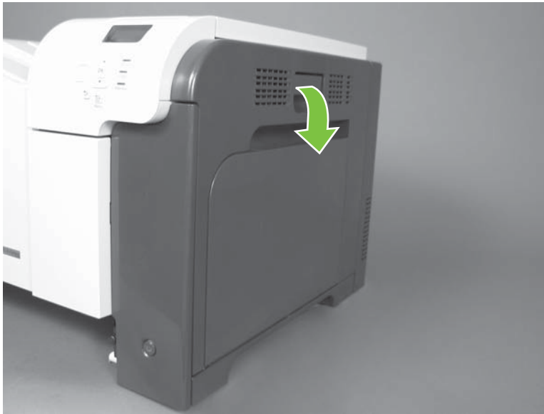
Figure 6-33 Remove the transfer roller (1 of 3)
