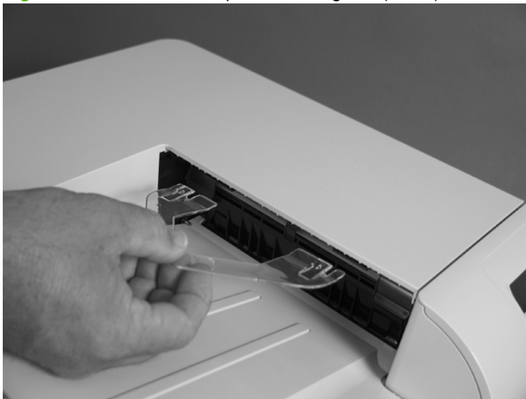
Figure 6-9 Remove the duplex-reverse guide (2 of 2)
