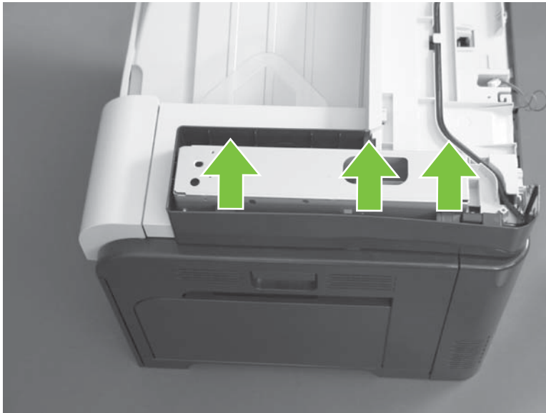
Figure 6-126 Remove the right-top cover (3 of 5)
