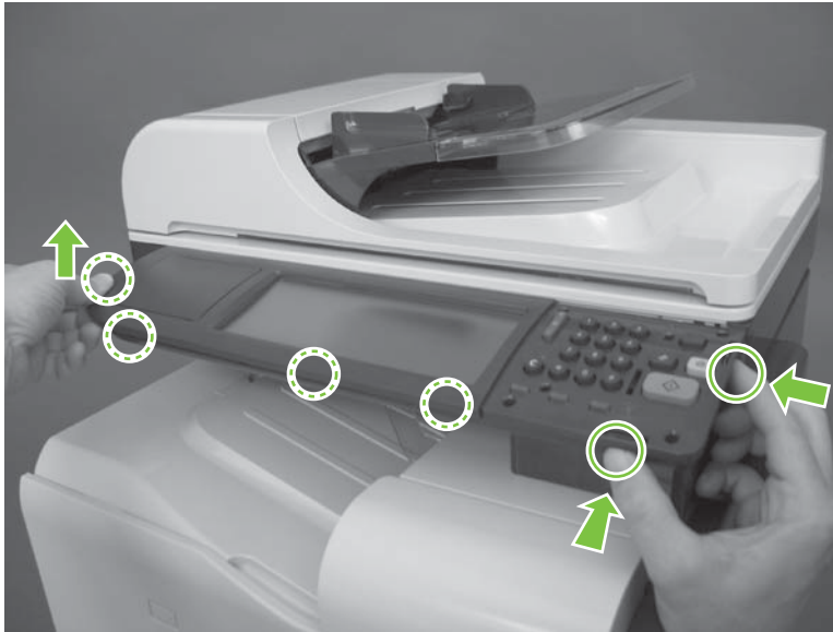
Figure 6-58 Remove the control-panel assembly (1 of 3)
