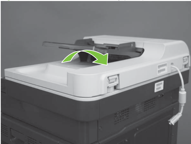
Figure 6-47 Remove the ADF assembly (2 of 4)
