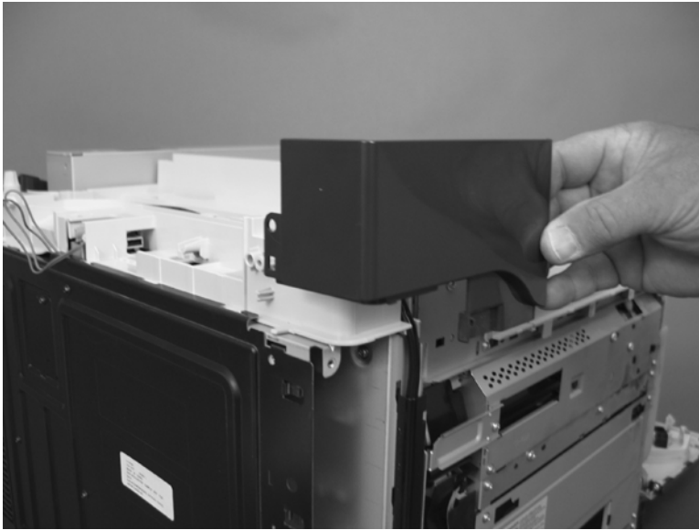
Figure 6-107 Remove the left-upper cover (2 of 2)
