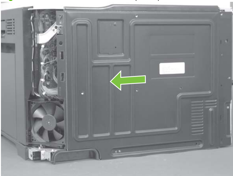
Figure 6-90 Remove the rear cover (2 of 2)
