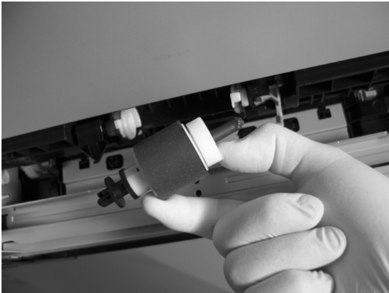
Figure 6-29 Remove the pickup roller (Tray 2) (4 of 4)
