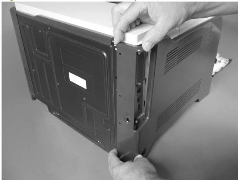
Figure 6-81 Remove the left cover (2 of 5)
