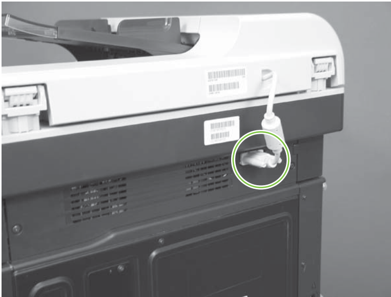
Figure 6-85 Remove the rear-upper cover (1 of 4)
