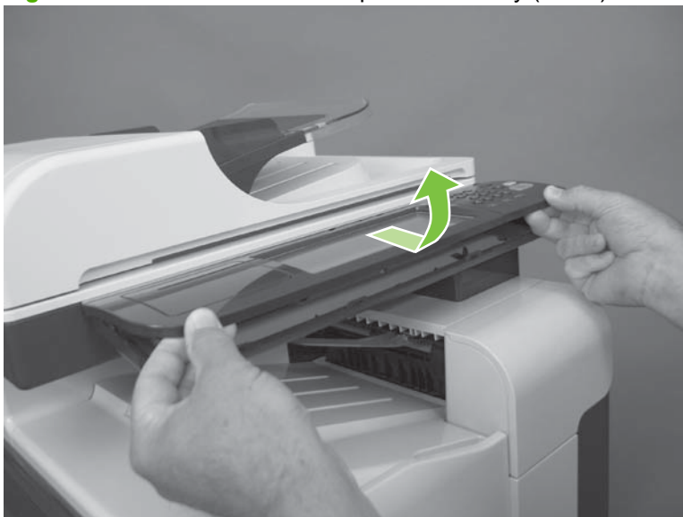
Figure 6-59 Remove the control-panel assembly (2 of 3)
