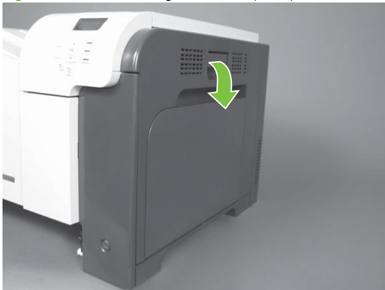
Figure 6-77 Remove the right-rear cover (1 of 3)
