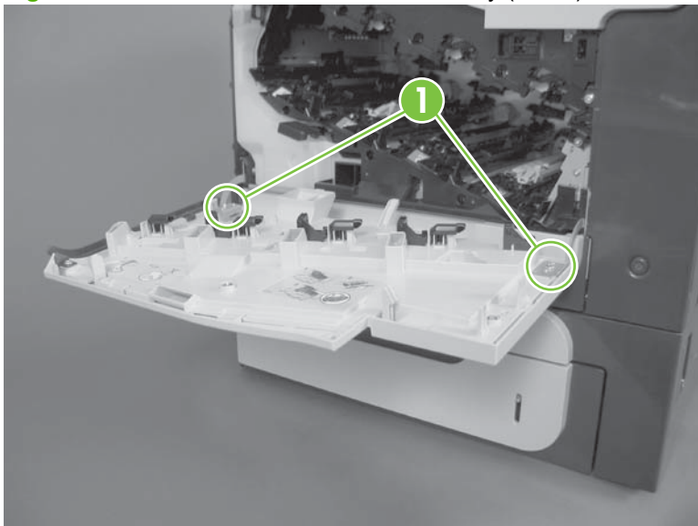
Figure 6-45 Remove the front-door assembly (2 of 2)
