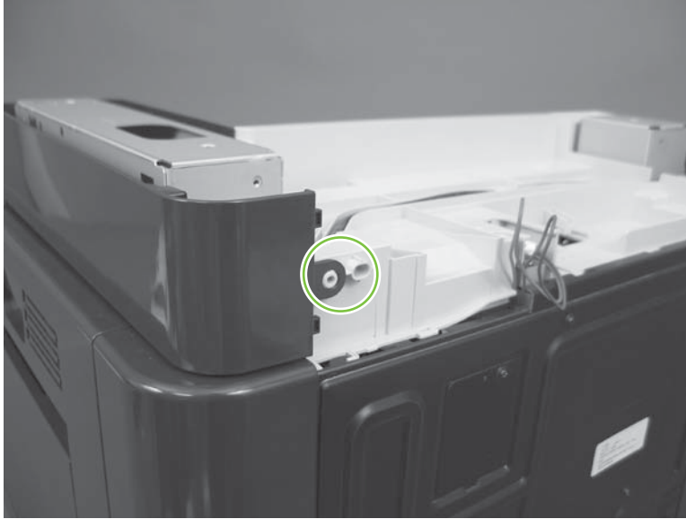
Figure 6-125 Remove the right-top cover (2 of 5)
