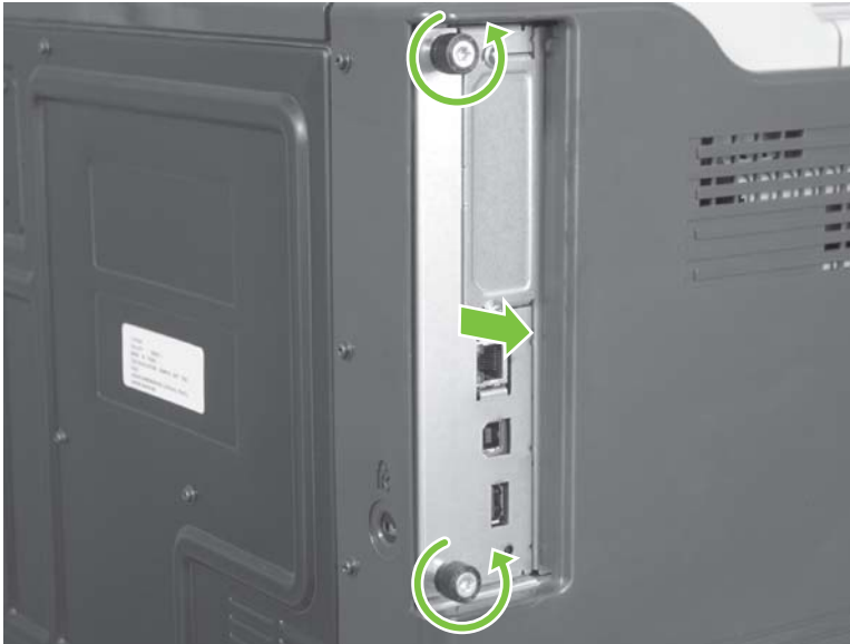
Figure 6-14 Remove the formatter
