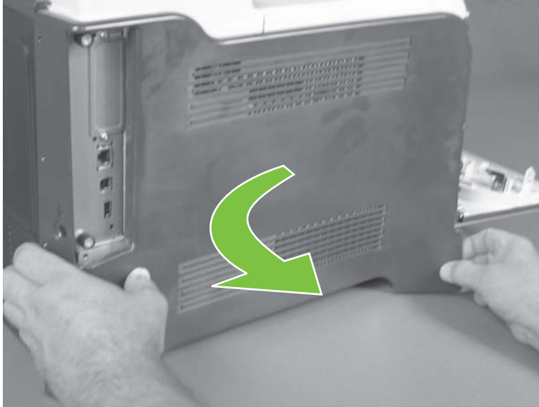
Figure 6-84 Remove the left cover (5 of 5)
