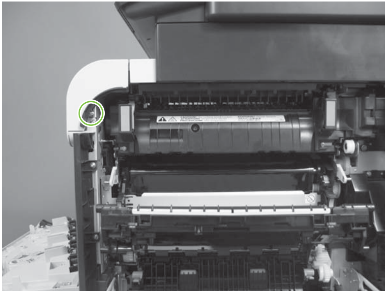
Figure 6-66 Remove the front-upper cover (2 of 4)
