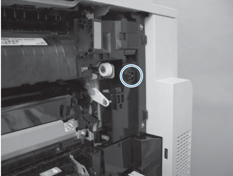
Figure 3-18 Test the right door switch
