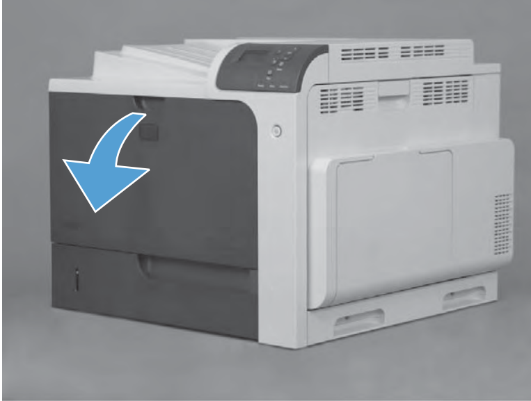
Figure 2-35 Remove the upper-left cover (1 of 3)
