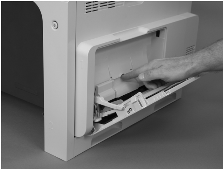
Figure 2-22 Remove the pickup roller (Tray 1) (2 of 5)
