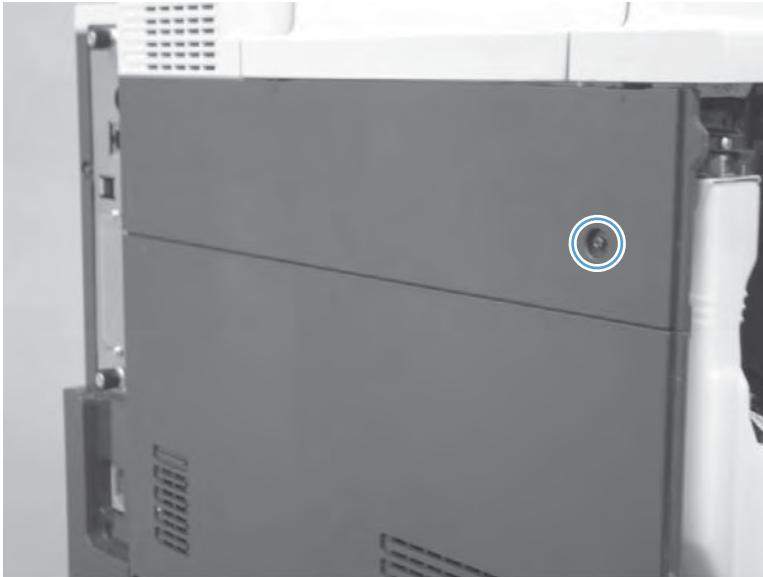
Figure 2-36 Remove the upper-left cover (2 of 3)
