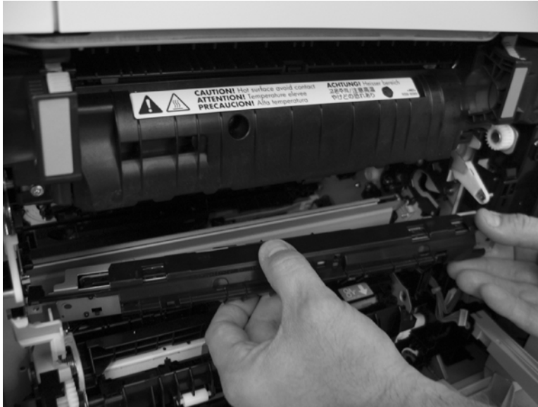
Figure 2-87 Remove the RD sensor assembly (7 of 7)
