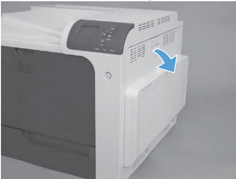
Figure 2-69 Remove the cassette feed guide (1 of 2)
