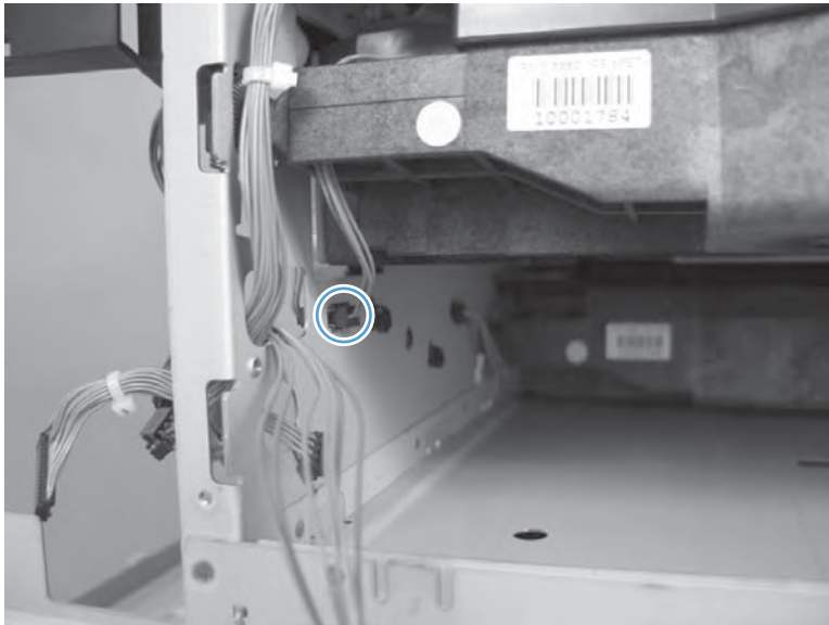
Figure 2-176 Remove the laser/scanner assembly (Y/M) (2 of 5)
