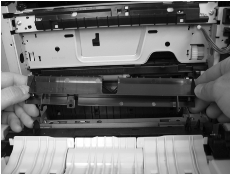
Figure 2-170 Remove the tray-pickup assembly (7 of 11)
