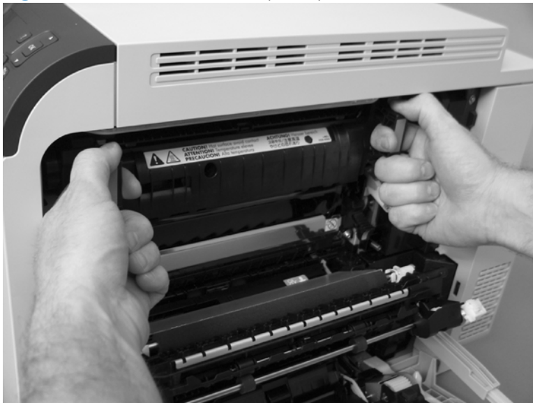
Figure 2-19 Remove the fuser (2 of 2)
