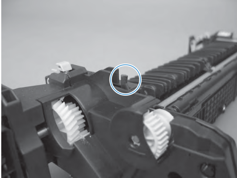
Figure 3-7 Test the fuser delivery sensor (1 of 2)
