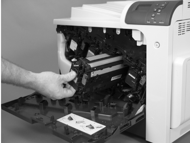
Figure 2-5 Remove the print cartridge (2 of 2)
