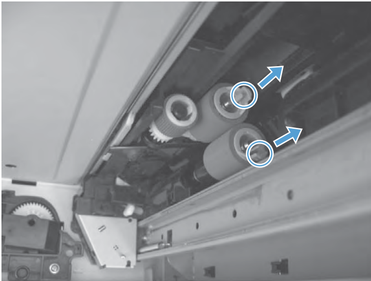
Figure 2-20 Remove the Pickup and feed rollers (Trays 2-5)
