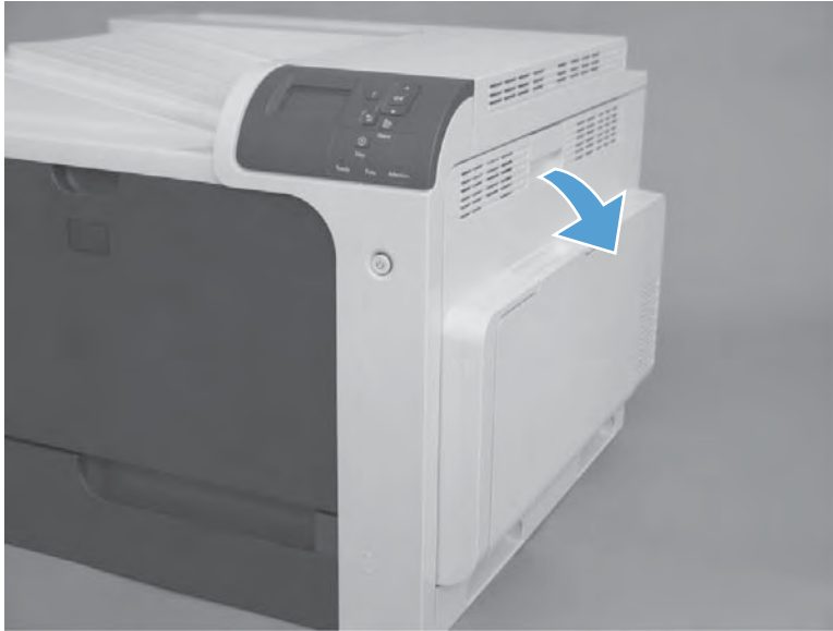
Figure 2-18 Remove the fuser (1 of 2)
