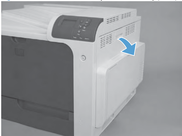
Figure 2-71 Remove the secondary transfer assembly (1 of 3)
