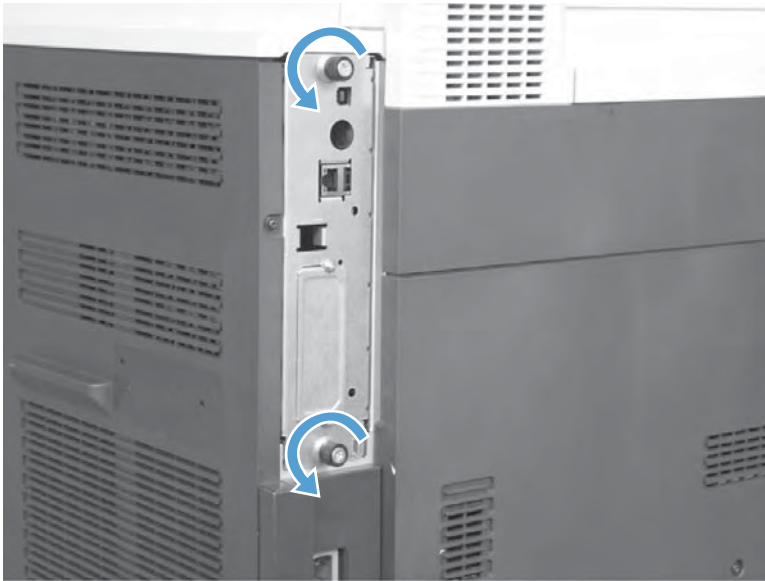
Figure 2-10 Remove the formatter
