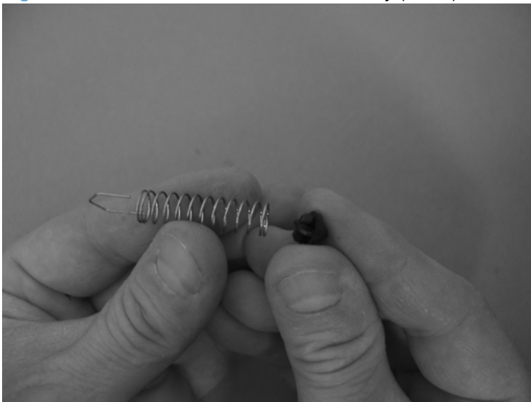
Figure 2-159 Reinstall the lifter base assembly (1 of 2)
