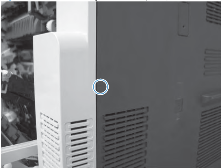
Figure 2-57 Remove the right-rear cover (1 of 2)
