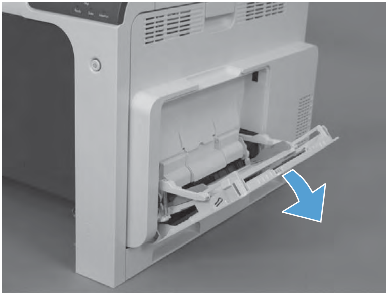
Figure 2-21 Remove the pickup roller (Tray 1) (1 of 5)
