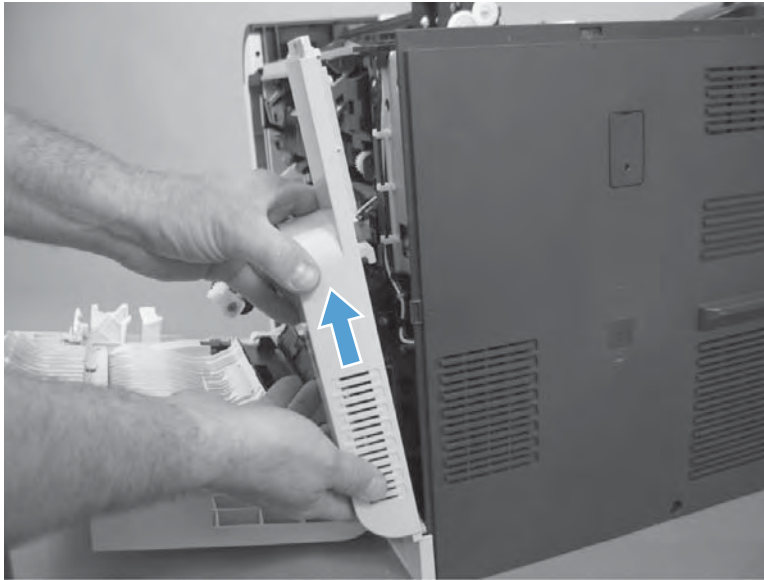
Figure 2-58 Remove the right-rear cover (2 of 2)
