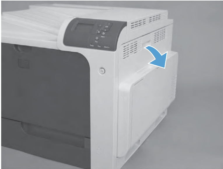
Figure 2-60 Remove the right-door assembly (1 of 9)
