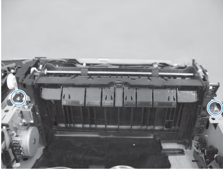
Figure 2-116 Remove the delivery assembly (4 of 7)
