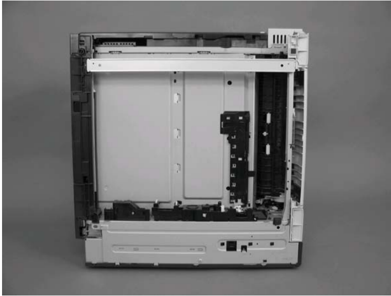
Figure 2-53 Remove the lifter-drive assembly (1 of 3)
