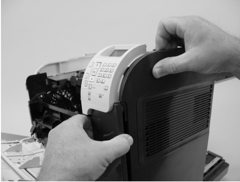
Figure 2-46 Remove the right-side cover (2 of 3)
