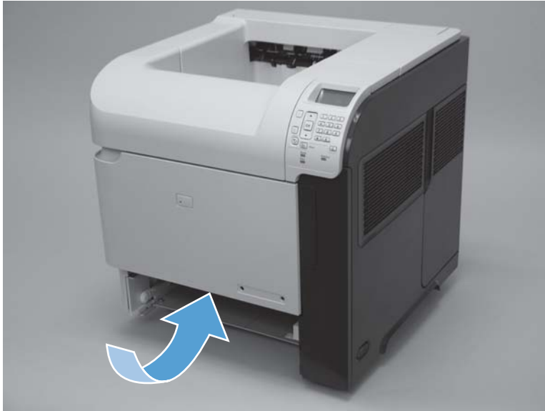
Figure 2-7 Remove the Tray 2 separation, pickup, and feed rollers (3 of 4)
