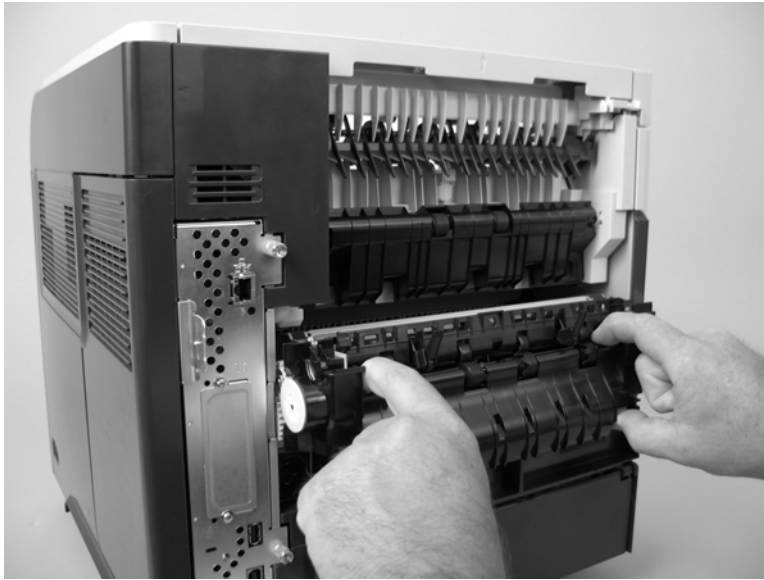
Figure 2-11 Remove the fuser (2 of 2)
