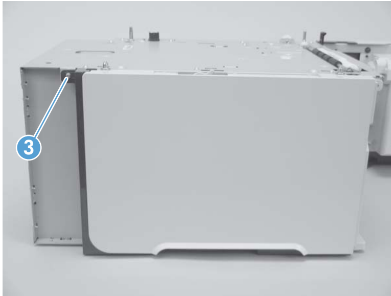
Figure 2-146 Remove the left-side cover (PD; 4 of 5)
