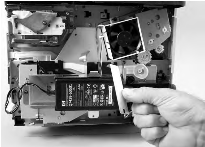
Figure 5-45 Remove the convenience-stapler power assembly (2 of 3)
