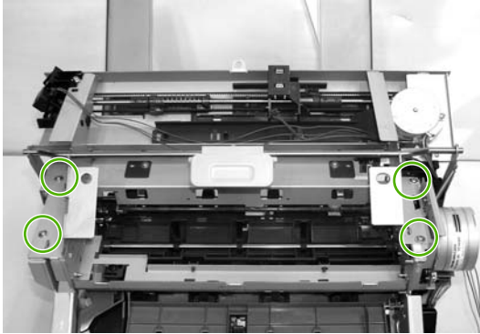
Figure 5-215 Remove the jogger unit (6 of 7)
