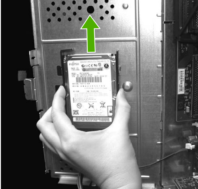
Figure 5-34 Remove the hard drive (2 of 2)
