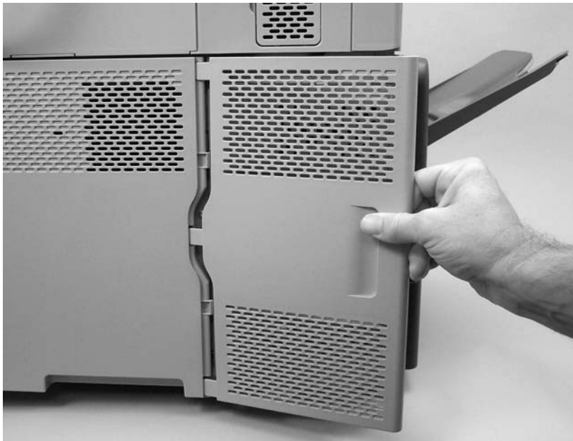
Figure 5-30 Remove the formatter cover and formatter (1 of 3)
