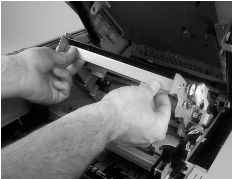
Figure 5-58 Remove the reversing assembly (8 of 8)
