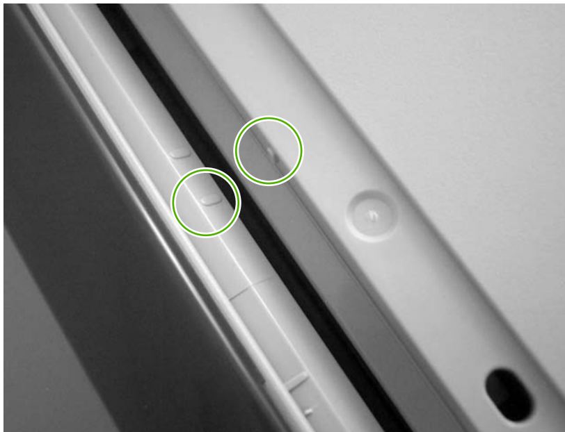
Figure 5-179 Correctly positioning the scanner assembly
