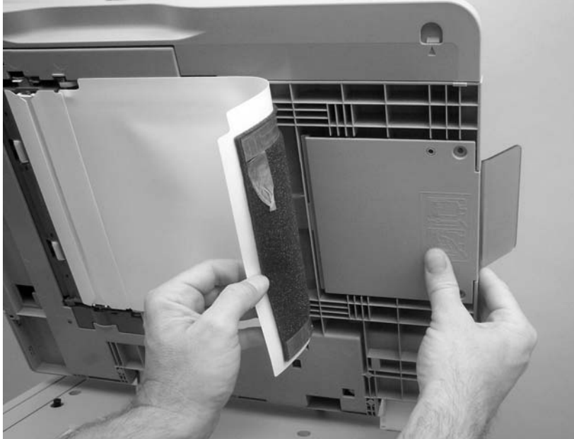
Figure 5-183 Remove the ADF output-bin extension (2 of 2)
