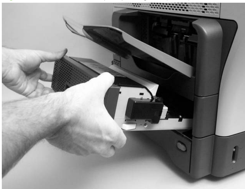
Figure 5-19 Remove the duplex-printing unit (2 of 2)
