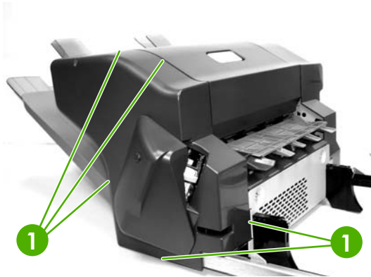
Figure 5-201 Claw locations on front cover
