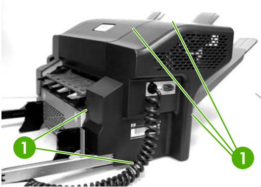
Figure 5-202 Claw locations on rear cover
