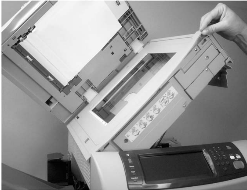
Figure 5-37 Remove the top-cover flatbed flange (1 of 2)
