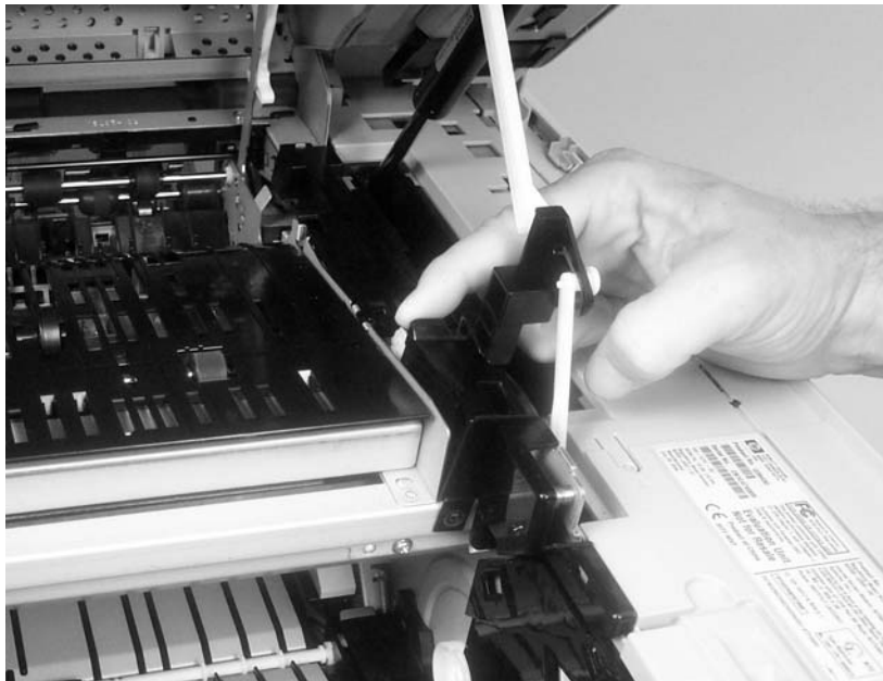
Figure 5-52 Remove the reversing assembly (2 of 8)
