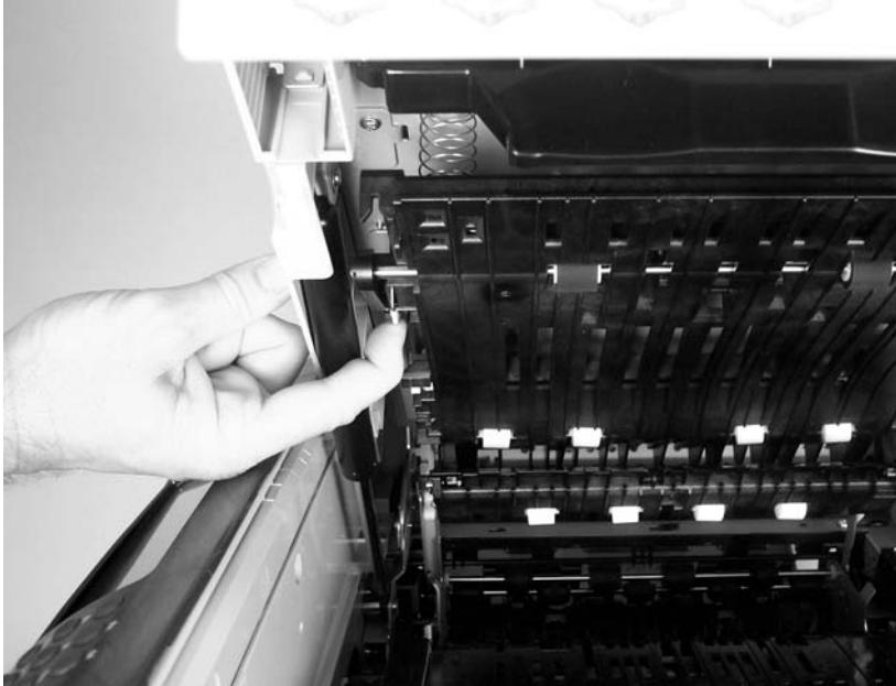
Figure 5-49 Remove the reversing-separation-guide assembly (1 of 2)
