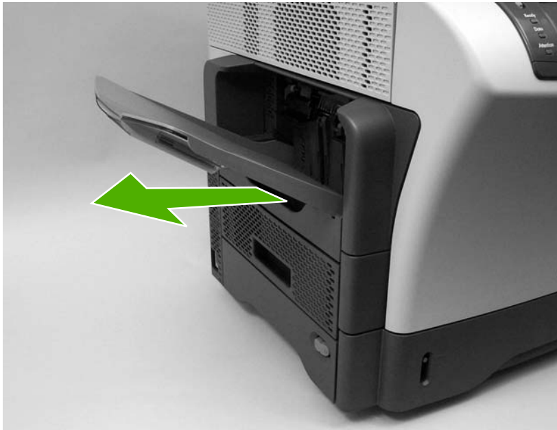
Figure 5-16 Remove the output-bin assembly (1 of 2)
