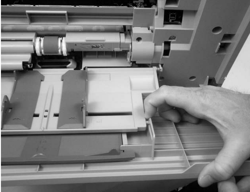
Figure 5-75 Remove the tray 1 assembly (1 of 5)
