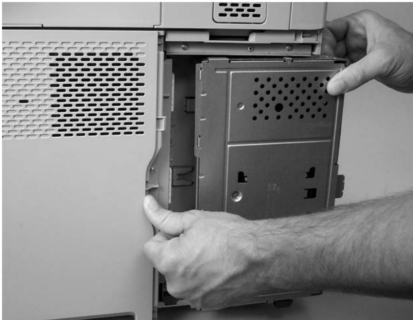
Figure 5-32 Remove the formatter cover and formatter (3 of 3)
