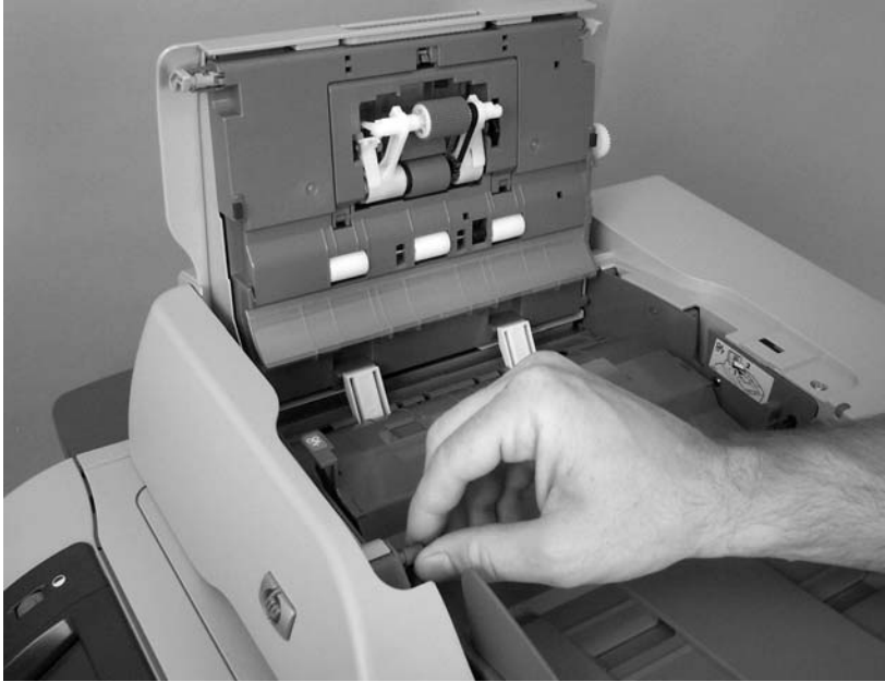
Figure 5-6 Remove the ADF input tray (2 of 3)
