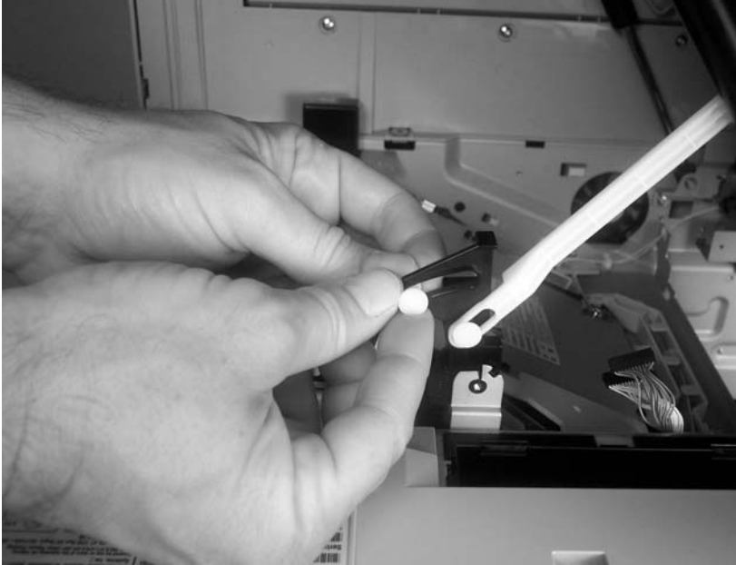
Figure 5-122 Remove the registration assembly (1 of 6)
