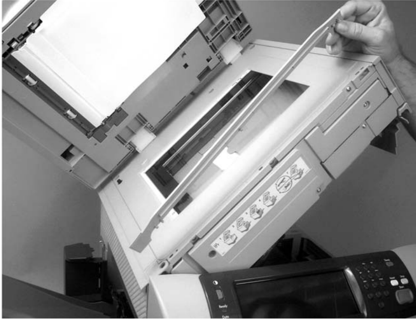
Figure 5-38 Remove the top-cover flatbed flange (2 of 2)
