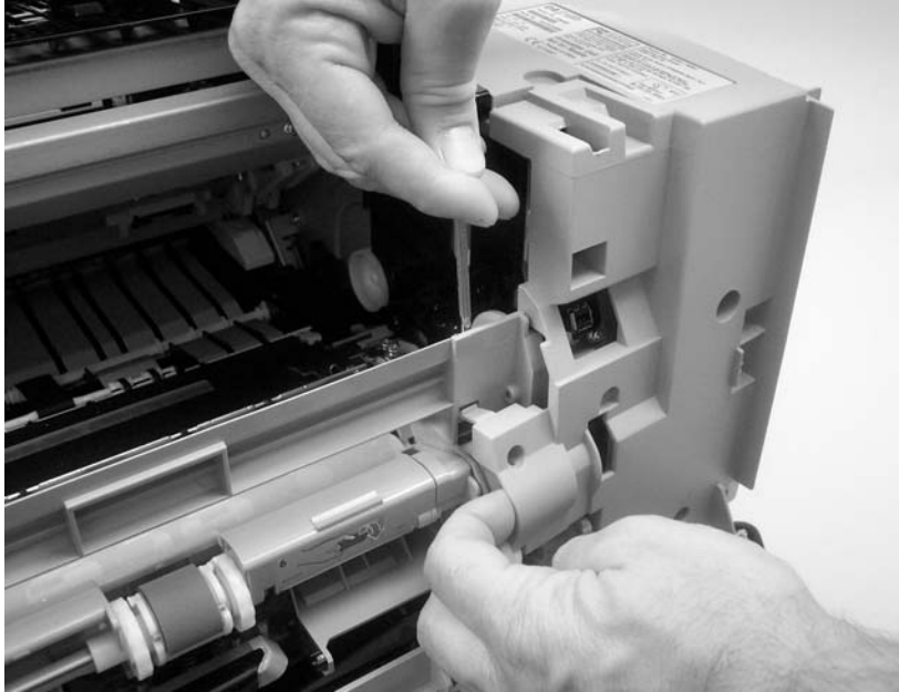
Figure 5-87 Remove the tray 1 feed-assembly (5 of 13)
