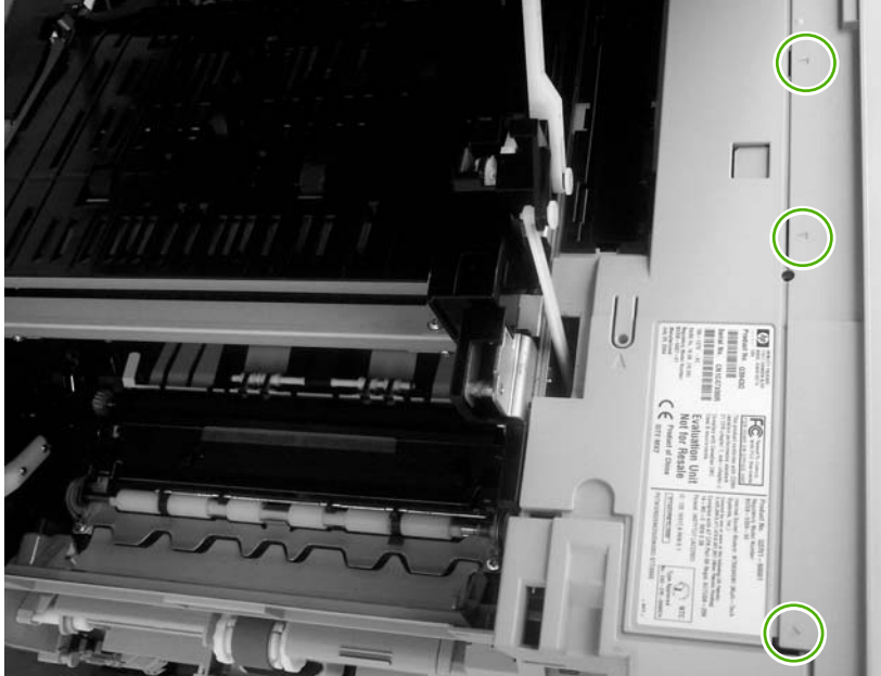
Figure 5-47 Remove the back cover (2 of 3)
