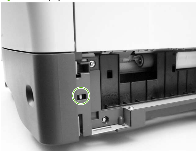
Figure 4-76 Tray 2 jam-access-cover switch, SW105
