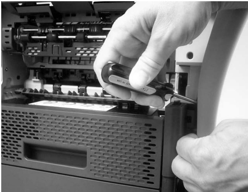
Figure 5-42 Remove the front cover (4 of 7)
