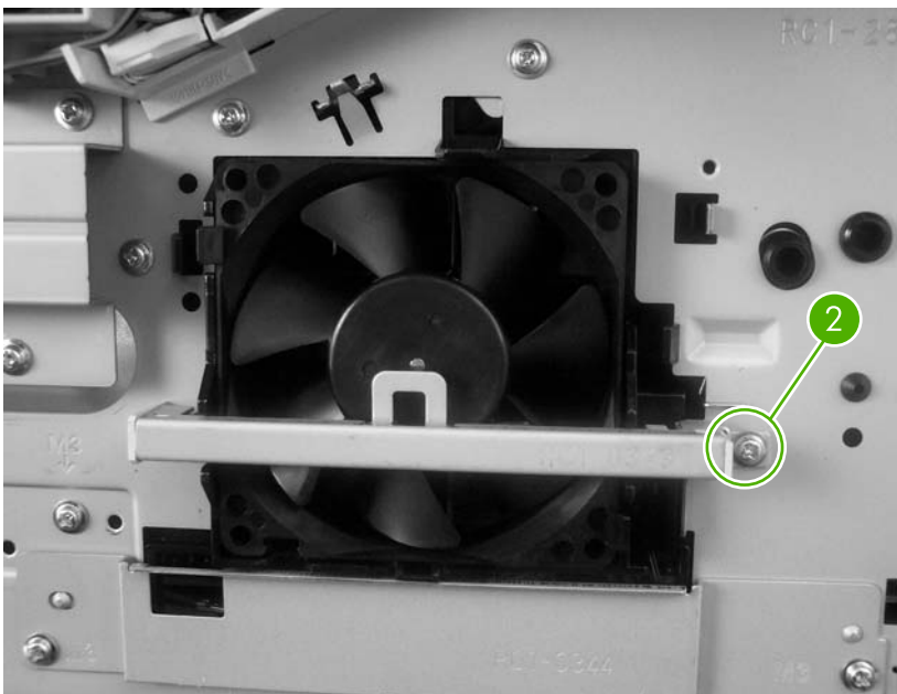
Figure 5-60 Remove the main fan and reversing-unit fan (2 of 9)
