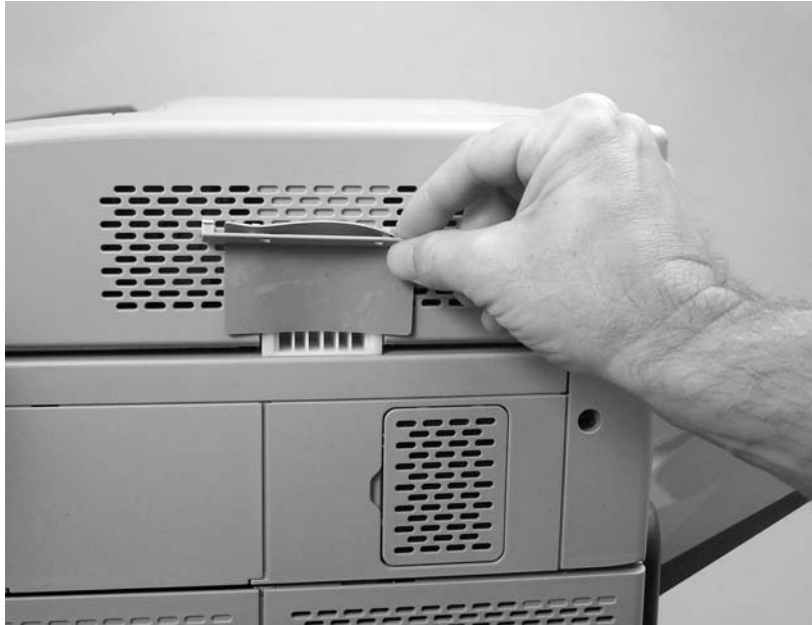
Figure 5-29 Remove the ADF-hinge flap (3 of 3)
