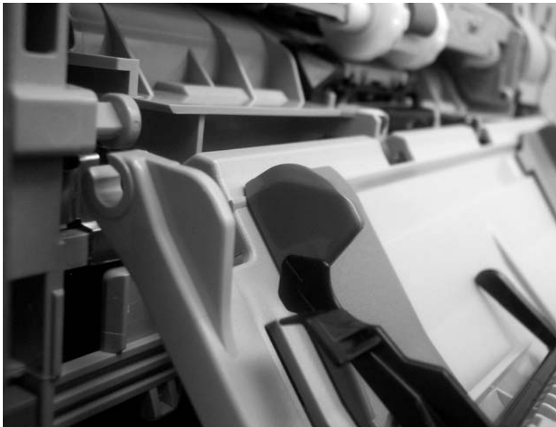
Figure 5-78 Remove the tray 1 assembly (4 of 5)
