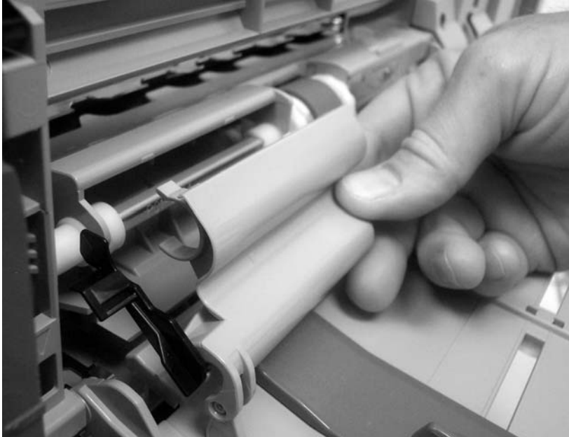
Figure 5-77 Remove the tray 1 assembly (3 of 5)
