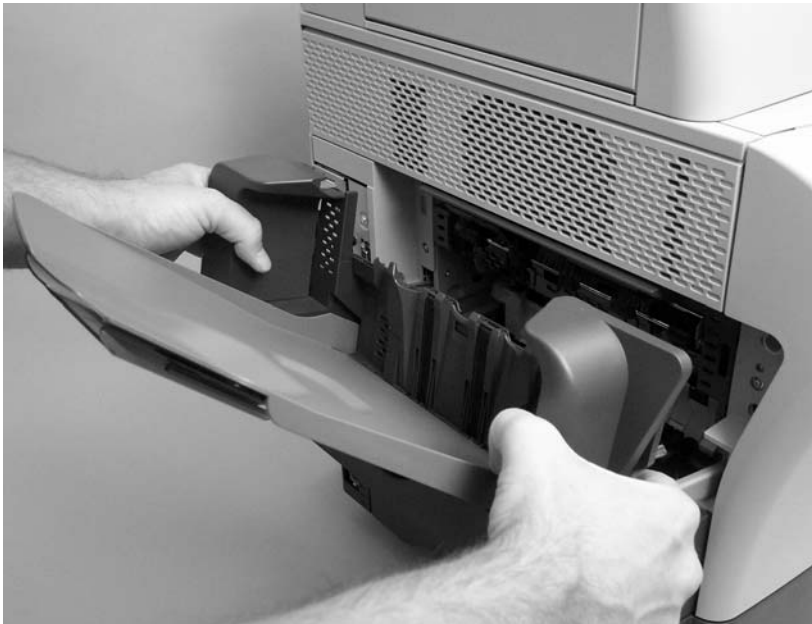
Figure 5-17 Remove the output-bin assembly (2 of 2)
