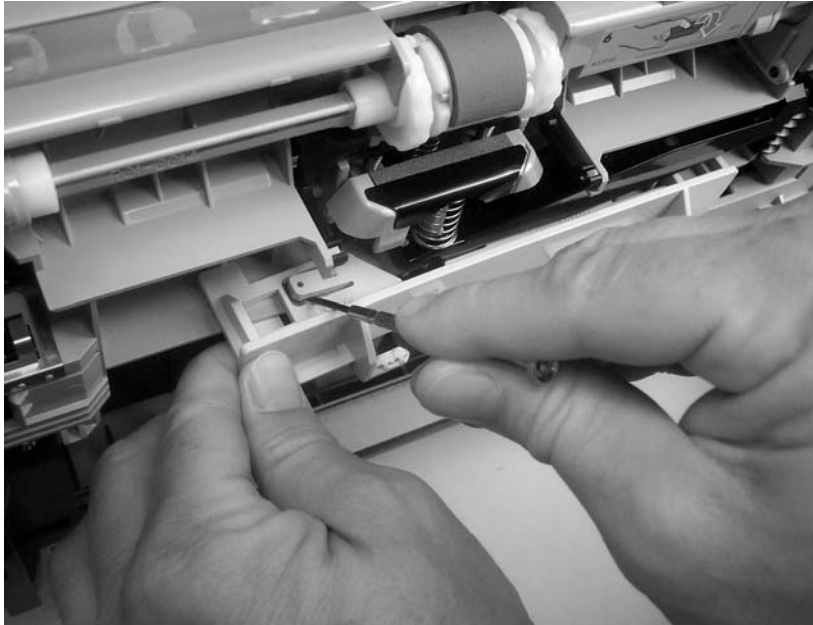
Figure 5-81 Remove the front-cover support (1 of 2)
