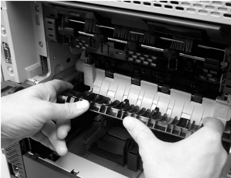
Figure 5-20 Remove the fuser-entrance guide
