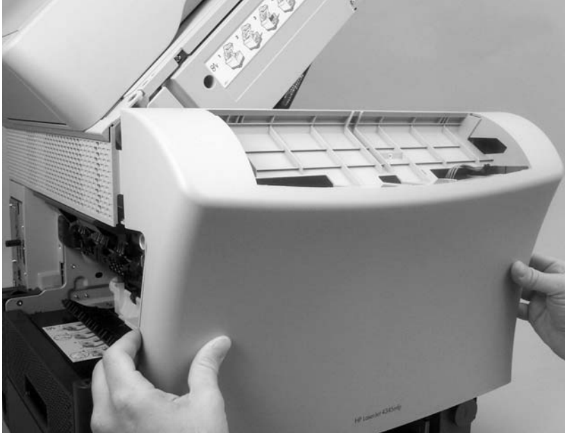
Figure 5-45 Remove the front cover (7 of 7)
