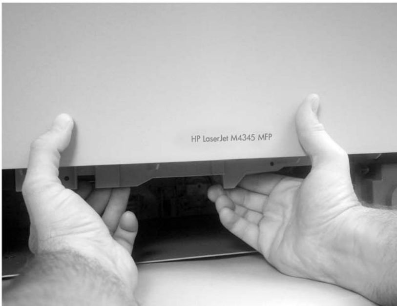
Figure 5-44 Remove the front cover (6 of 7)
