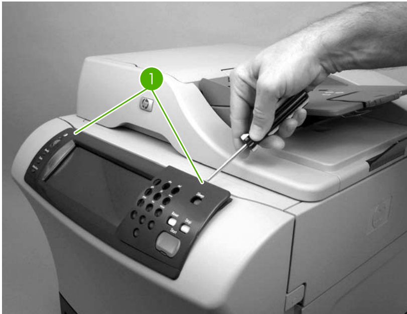
Figure 5-1 Remove the control-panel overlays
