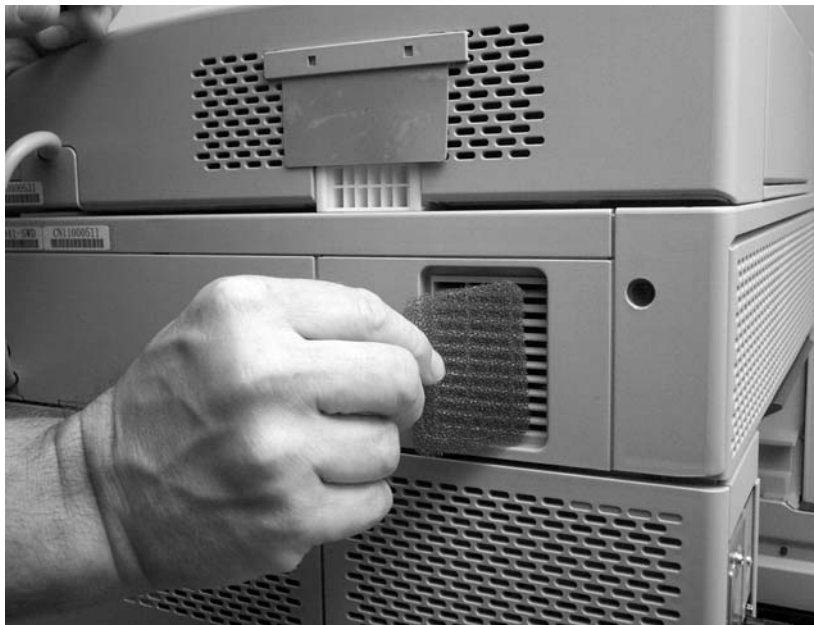
Figure 5-26 Remove the scanner filter (2 of 2)
