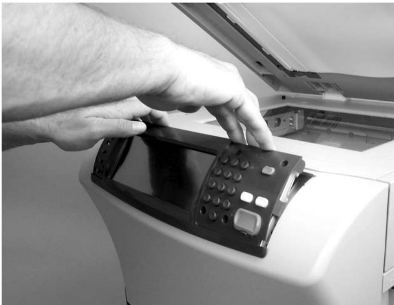
Figure 5-2 Remove the control panel (1 of 2)
