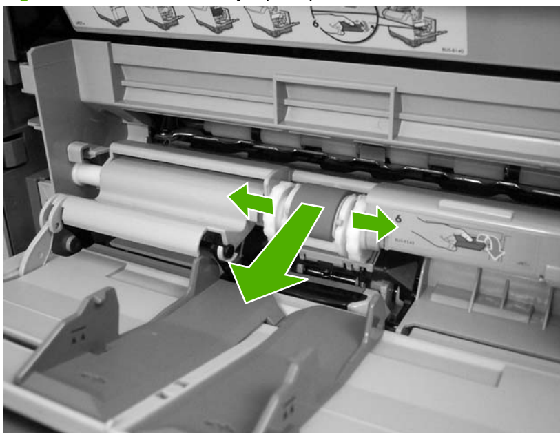
Figure 5-24 Remove the tray 1 pickup roller
