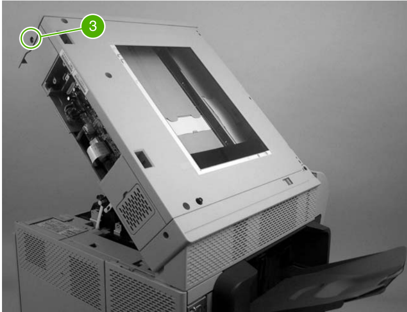
Figure 5-173 Remove the scanner assembly (3 of 8)
