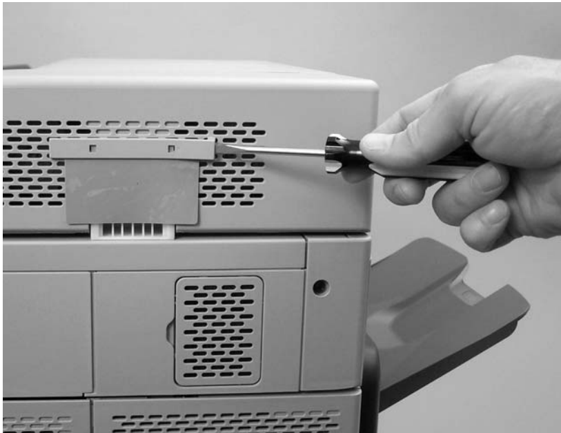
Figure 5-27 Remove the ADF-hinge flap (1 of 3)
