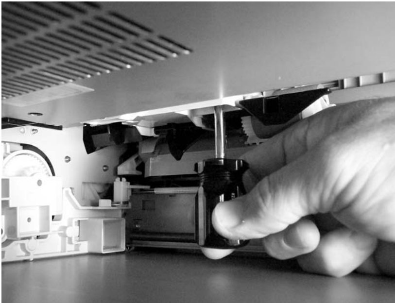
Figure 5-162 Remove the tray 2 paper-present sensor
