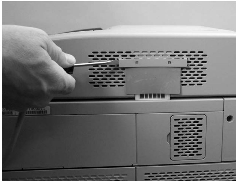
Figure 5-28 Remove the ADF-hinge flap (2 of 3)
