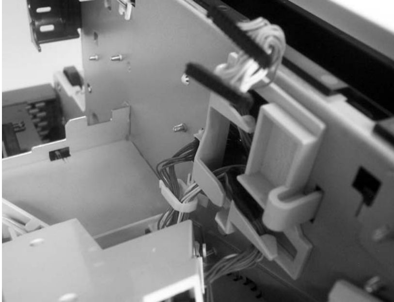
Figure 5-164 Remove the laser/scanner (1 of 2)
