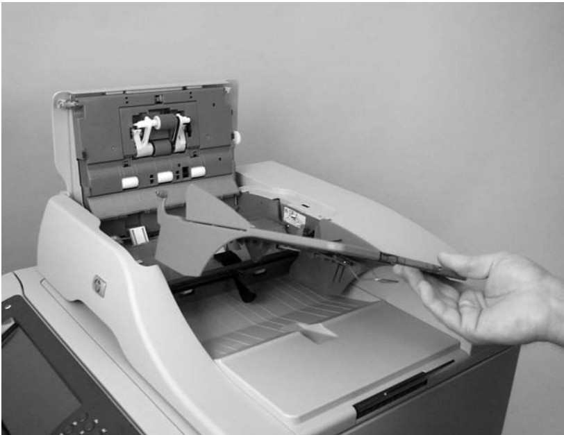
Figure 5-7 Remove the ADF input tray (3 of 3)
