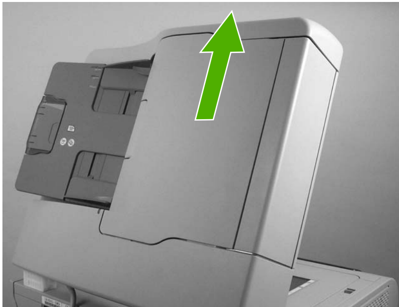
Figure 5-170 Remove the ADF assembly (3 of 3)
