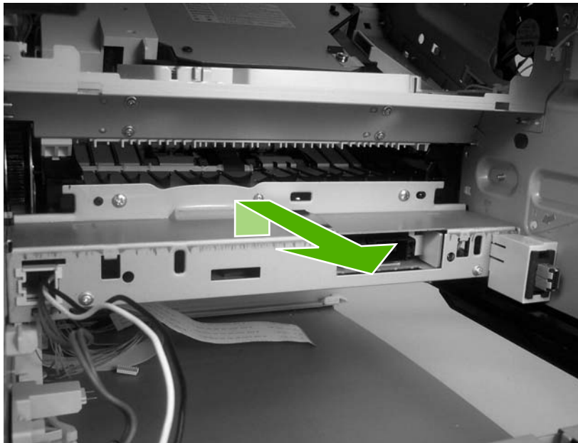
Figure 5-157 Remove the engine power supply (10 of 10)
