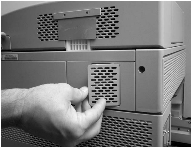
Figure 5-25 Remove the scanner filter (1 of 2)
