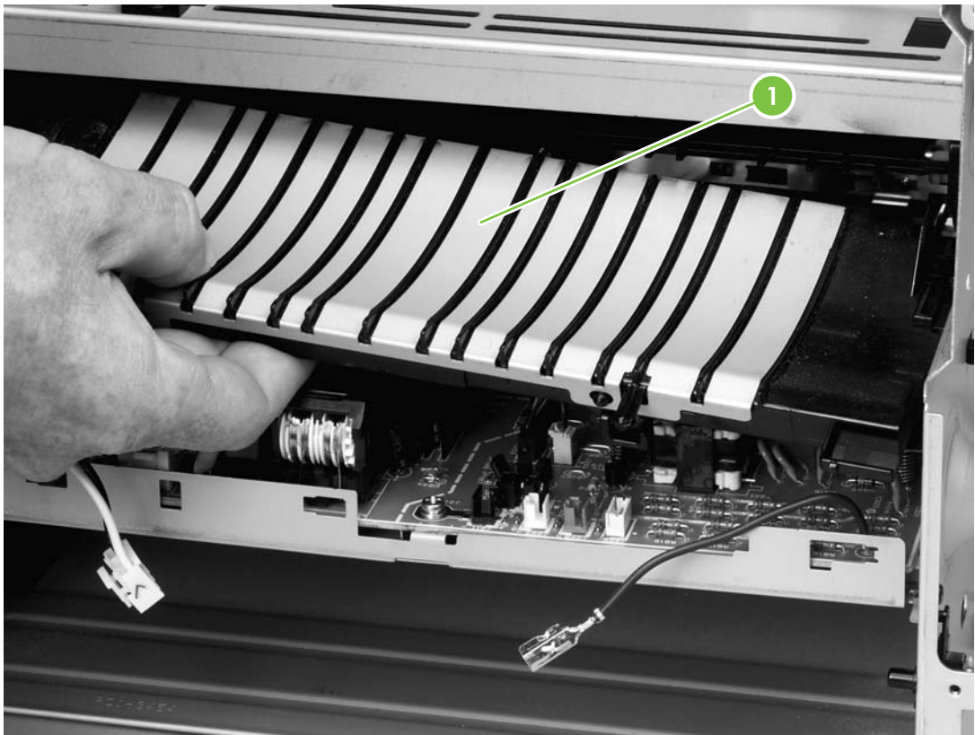
Figure 6-27 Removing the ECU (1 of 7)
