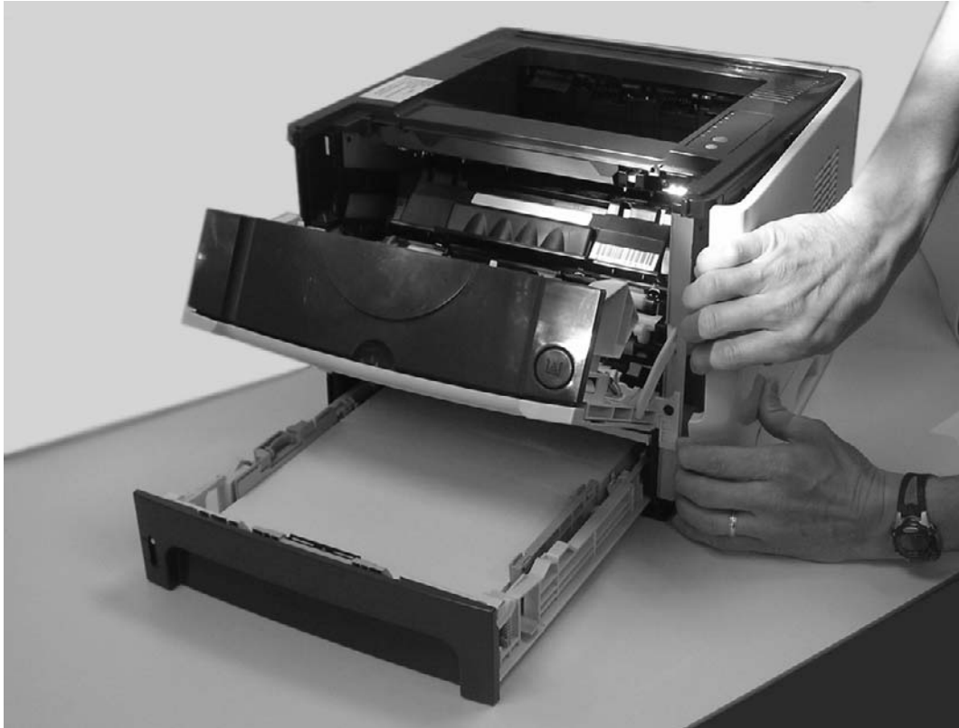
Figure 6-2 Removing the right-side cover
