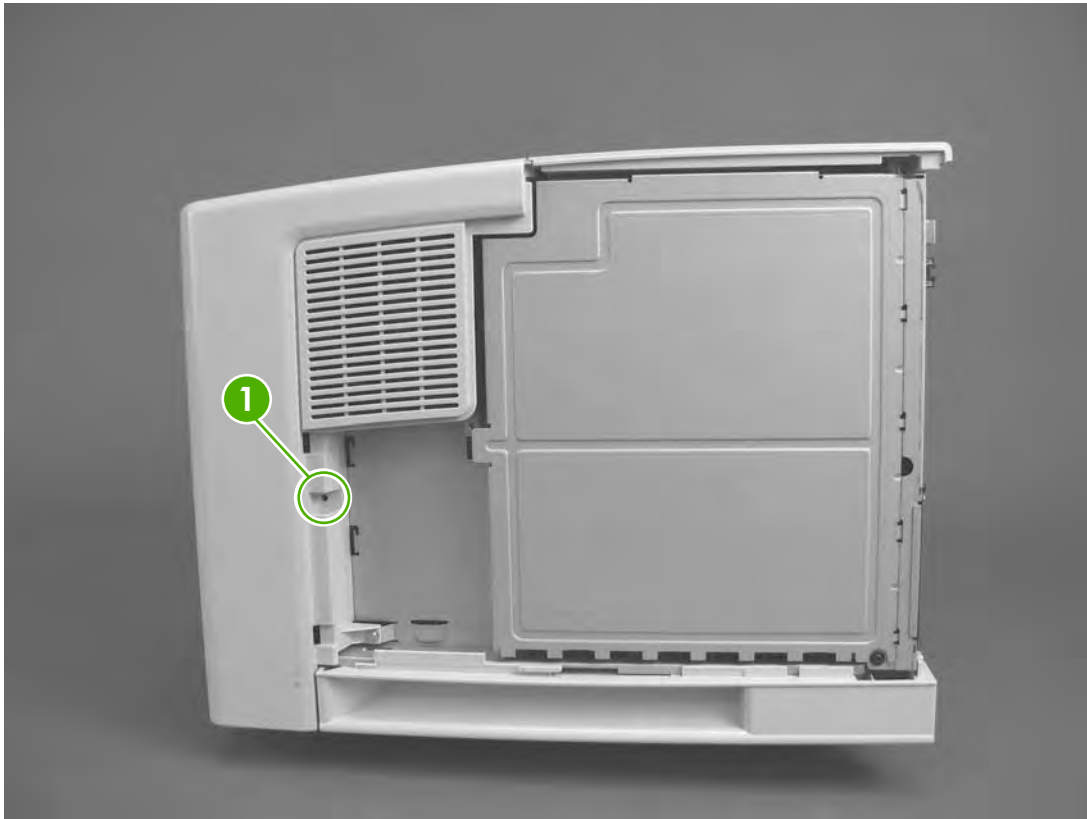
Figure 6-3 Locating the engine-test-page switch
