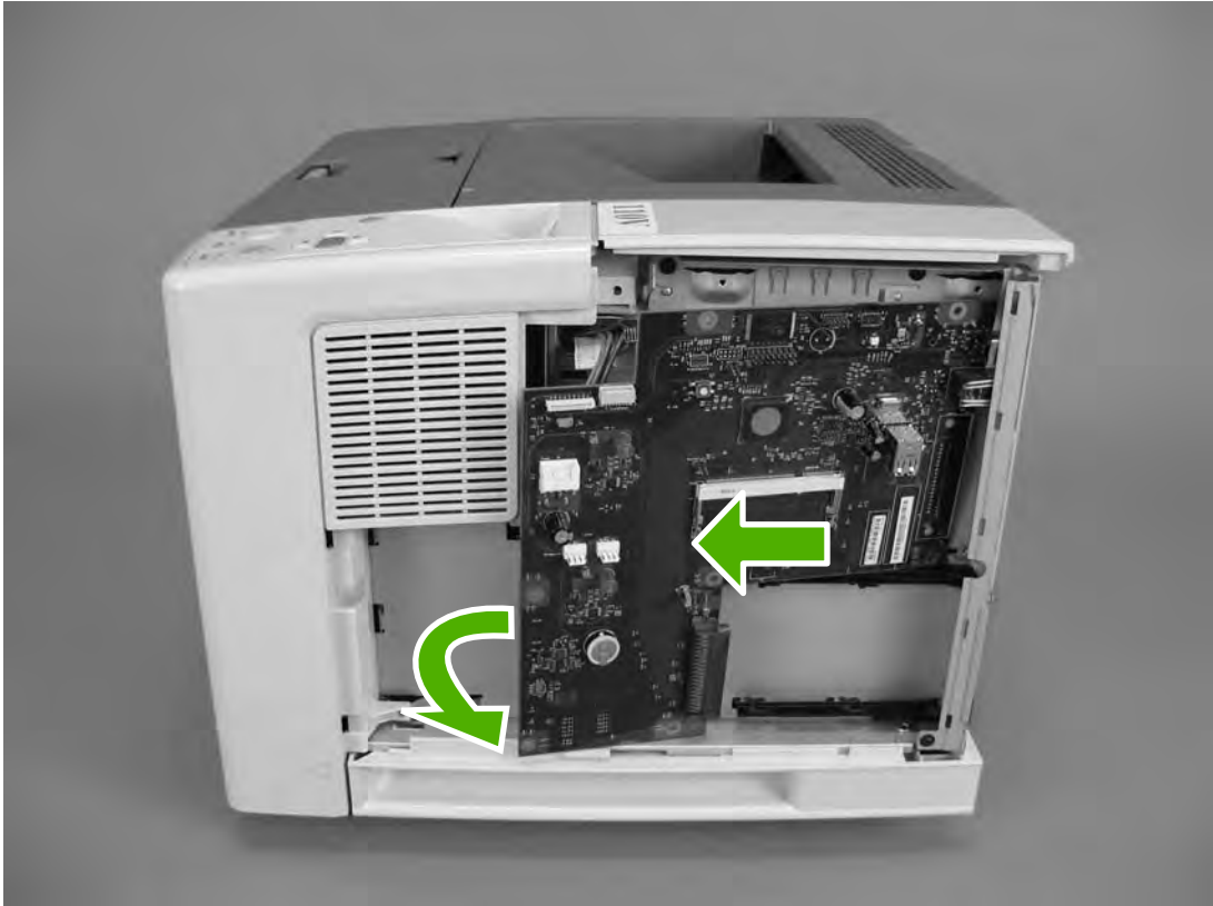
Figure 5-15 Removing the formatter (3 of 3)
