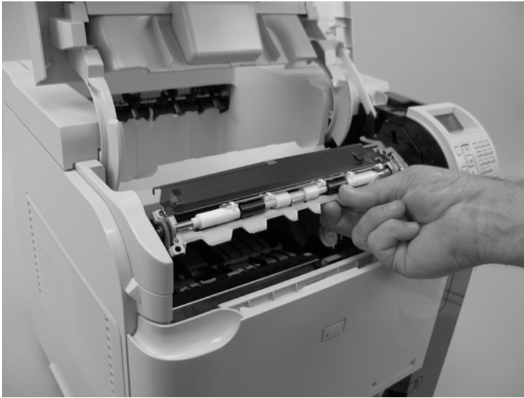
Figure 6-36 Remove the registration assembly (3 of 4)
