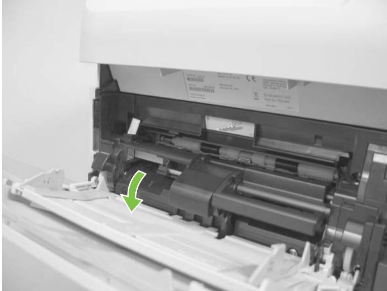
Figure 6-31 Remove the Tray 1 separation roller (1 of 3)
