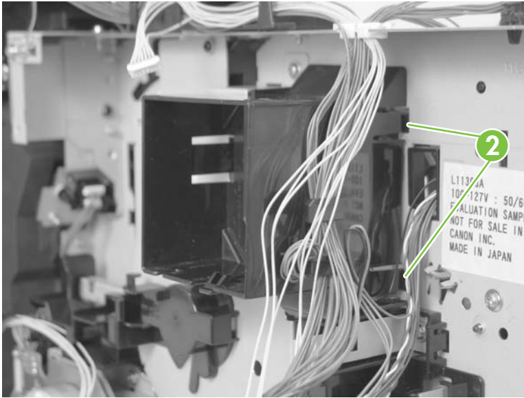
Figure 6-91 Remove the drum-drive assembly (2 of 4)
