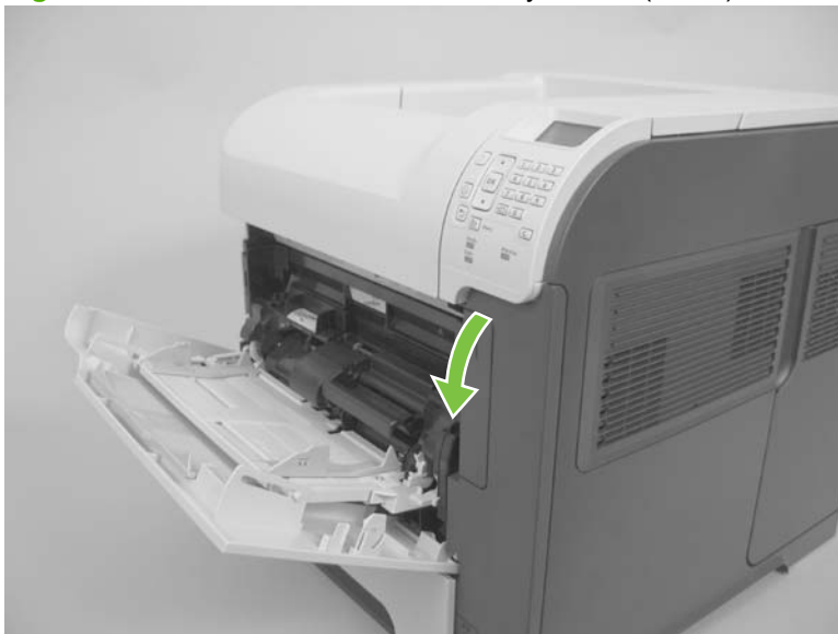
Figure 6-16 Remove the front accessory covers (2 of 2)
