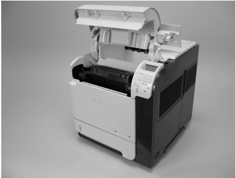
Figure 6-5 Remove the print cartridge (1 of 2)
