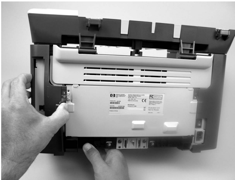
Figure 6-9 Remove the scanner assembly (2 of 11)
