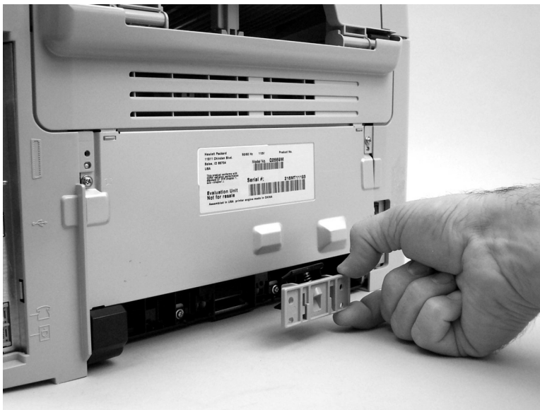
Figure 6-20 Remove the device separation pad (2 of 2)
