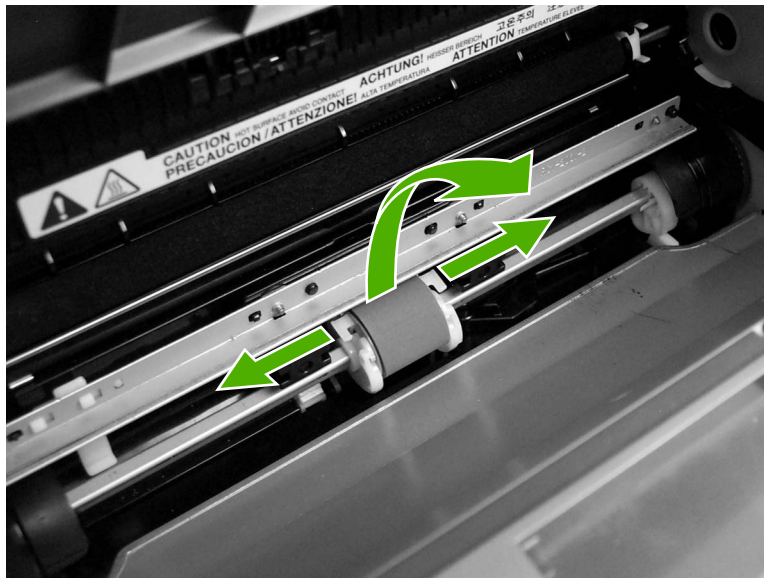
Figure 6-24 Remove the device pickup roller (2 of 5)
