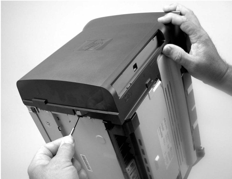
Figure 6-10 Remove the scanner assembly (3 of 11)
