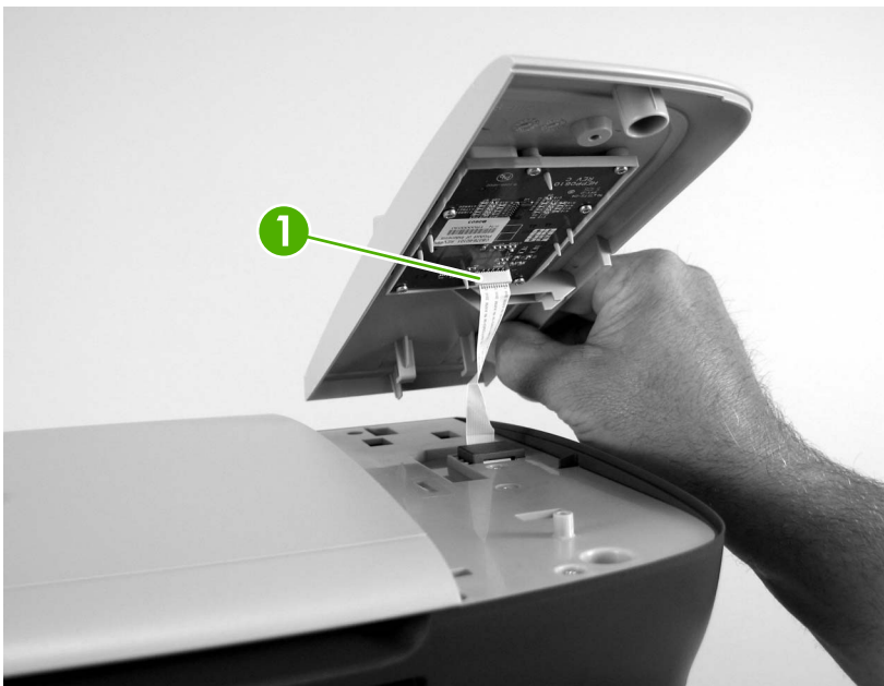
Figure 6-7 Remove the control panel (4 of 4)
