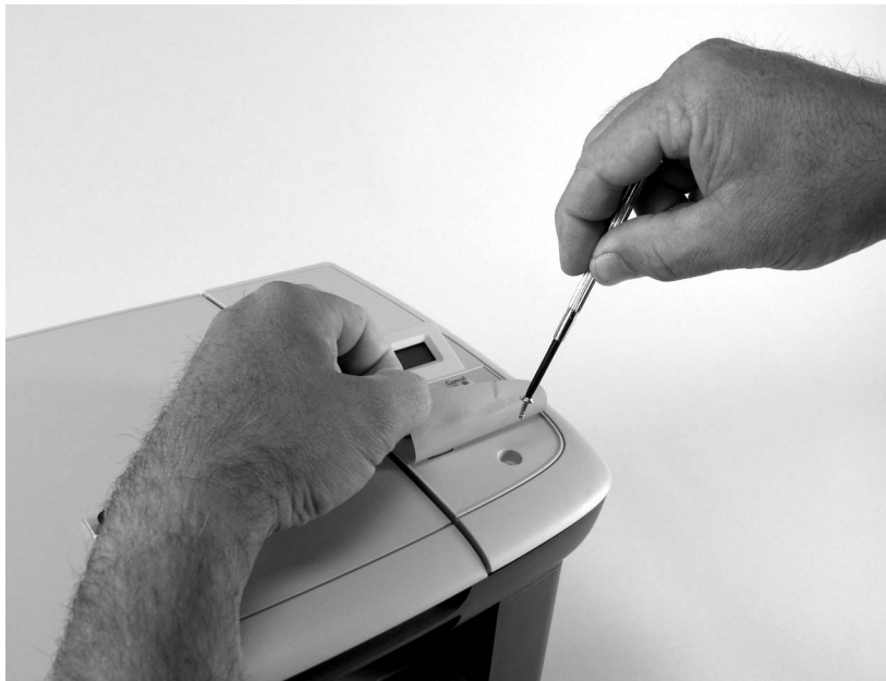
Figure 6-5 Remove the control panel (2 of 4)
