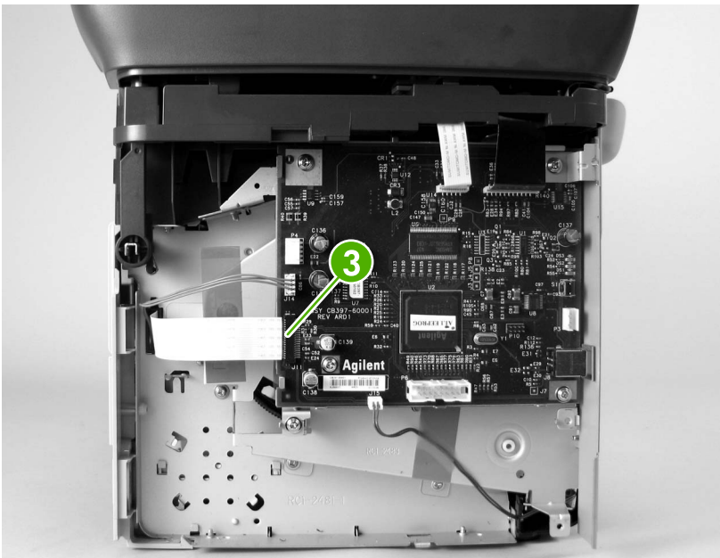
Figure 6-58 Remove the ECU (3 of 6)
