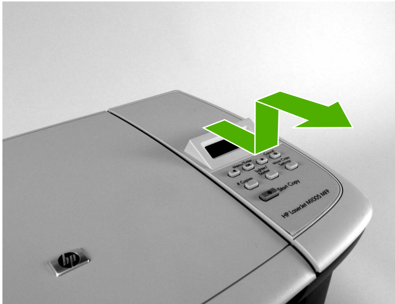
Figure 6-6 Remove the control panel (3 of 4)
