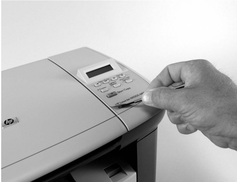
Figure 6-3 Remove the control-panel overlay
