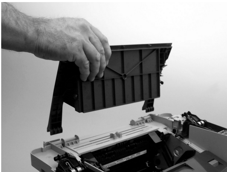
Figure 6-39 Remove the print-cartridge door (2 of 2)
