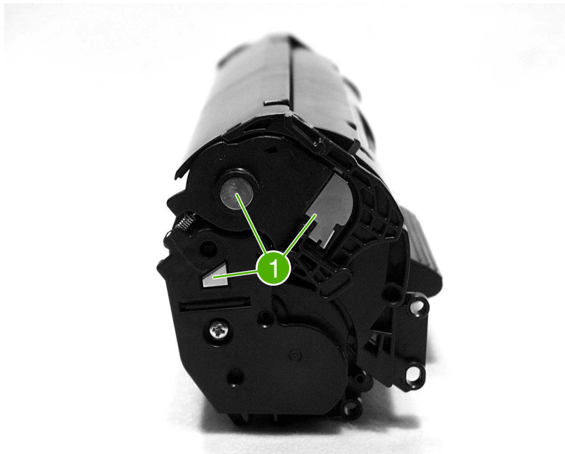
Figure 7-7 Print-cartridge high-voltage contacts
