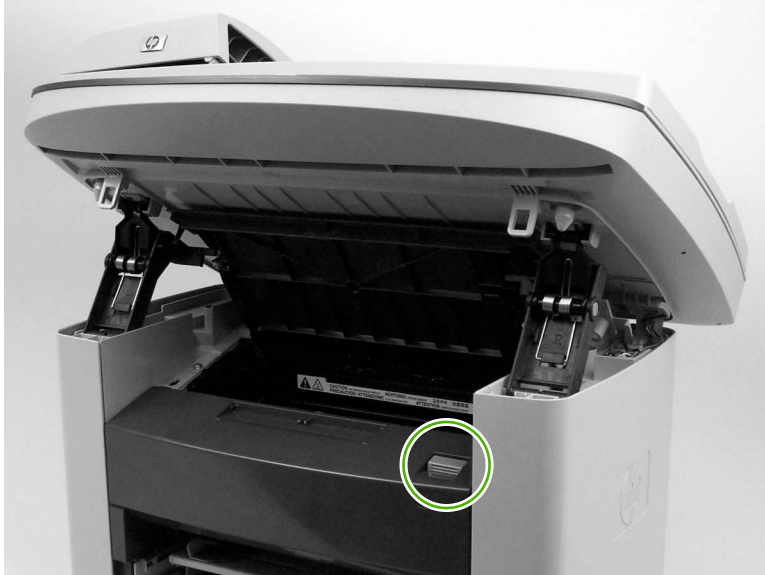
Figure 6-21 Remove the print cartridge (1 of 2)
