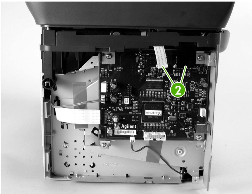
Figure 6-11 Remove the scanner assembly (4 of 11)
