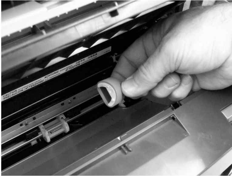
Figure 6-25 Remove the device pickup roller (3 of 5)
