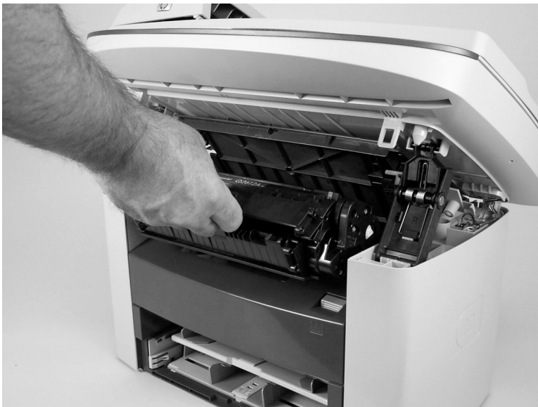
Figure 6-22 Remove the print cartridge (2 of 2)
