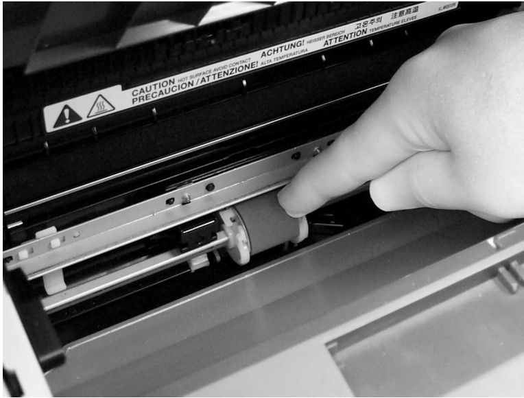
Figure 6-27 Remove the device pickup roller (5 of 5)
