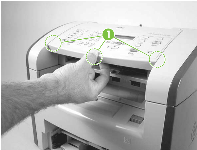
Figure 6-11 Removing the top cover, control panel (1 of 3)
