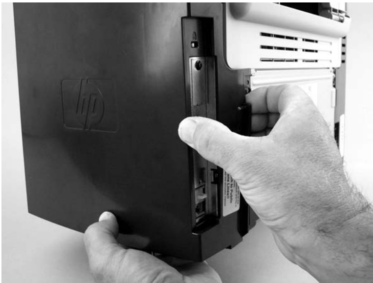
Figure 6-23 Removing the scanner assembly (4 of 14)
