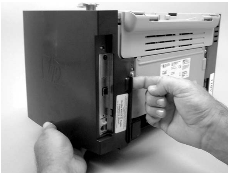
Figure 6-62 Removing the side covers (2 of 4)
