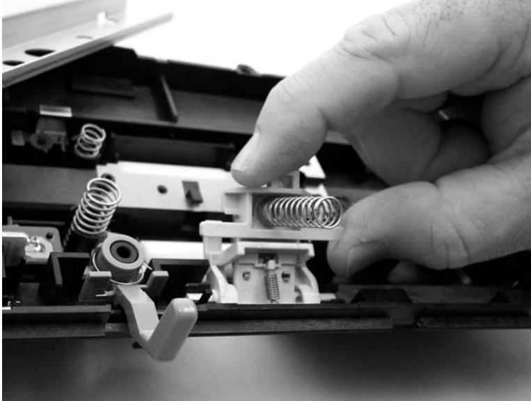
Figure 6-18 Removing the separation-pad assembly (2 of 3)
