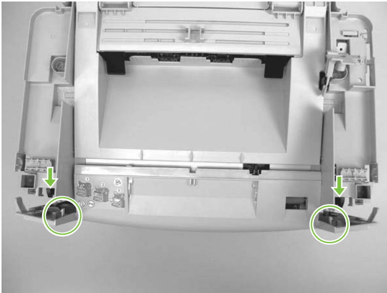
Figure 6-73 Removing the front cover (4 of 5)
