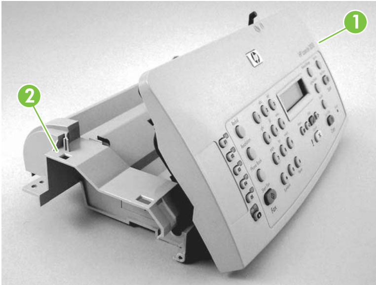
Figure 6-38 Removing the top-cover assembly (1 of 2)
