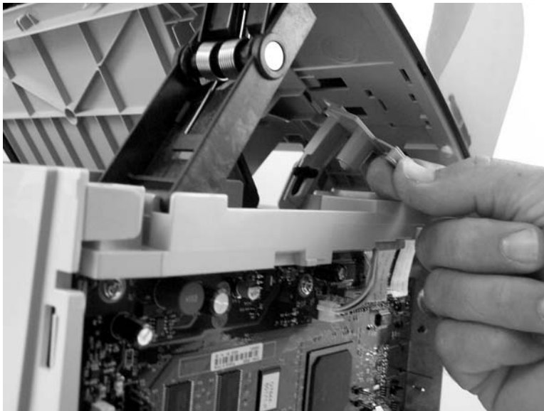
Figure 6-29 Removing the scanner assembly (10 of 14)
