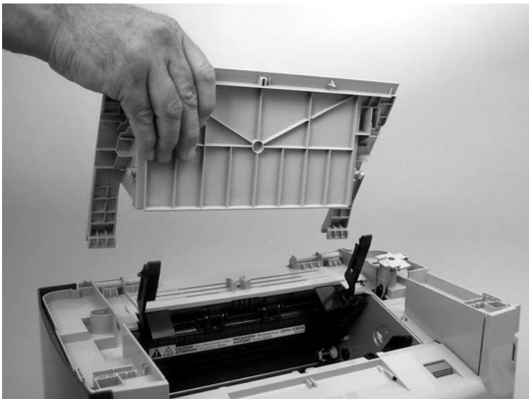
Figure 6-66 Removing the print-cartridge door (2 of 2)
