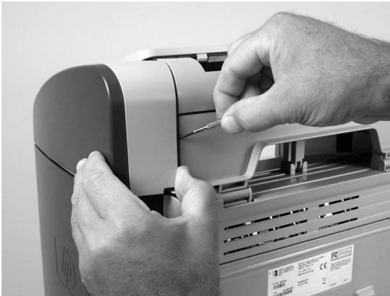
Figure 6-8 Removing the scanner side covers (1 of 2)
