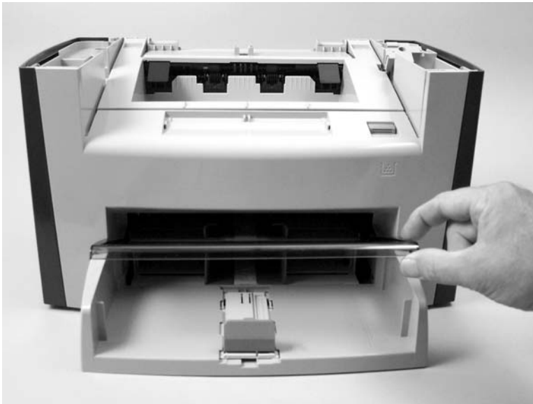
Figure 6-55 Removing the media input tray (1 of 3)
