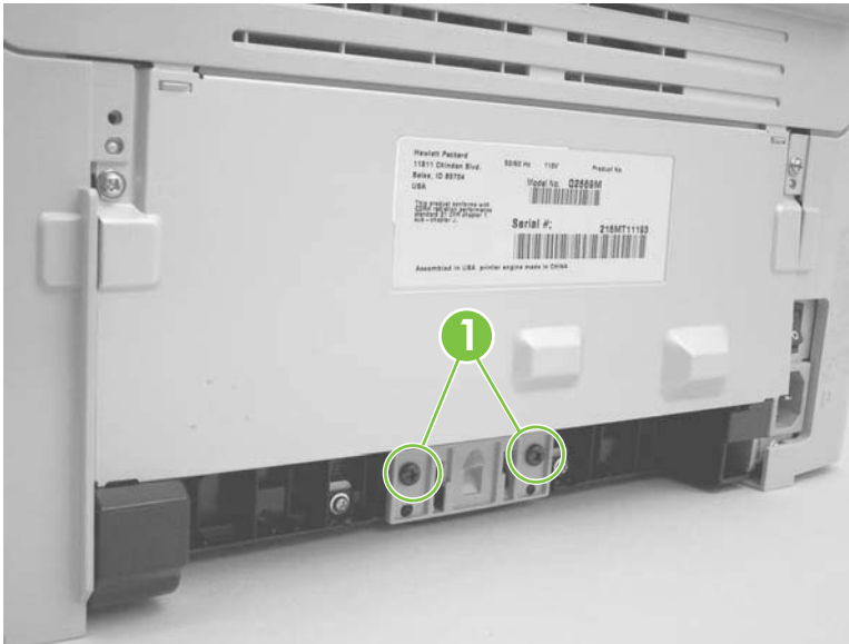
Figure 6-45 Removing the separation pad (1 of 2)
