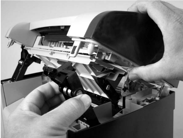
Figure 6-5 Removing the link assemblies and scanner support-frame spring (2 of 4)
