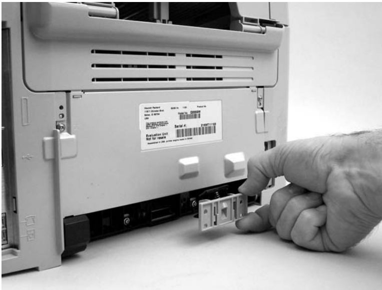
Figure 6-46 Removing the separation pad (2 of 2)
