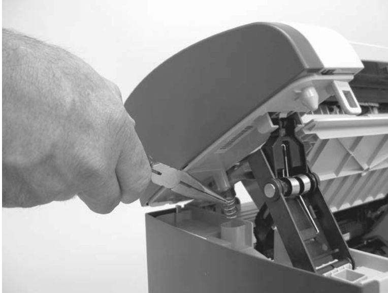
Figure 6-7 Removing the link assemblies and scanner support-frame spring (4 of 4)
