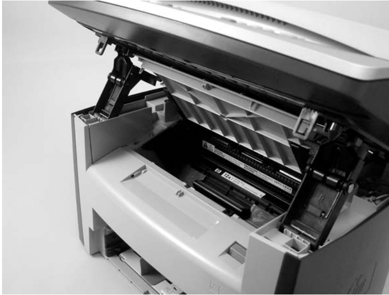
Figure 6-47 Removing the print cartridge (1 of 2)
