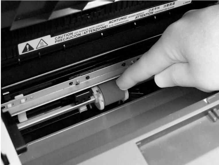
Figure 6-53 Removing the pickup roller (5 of 5)
