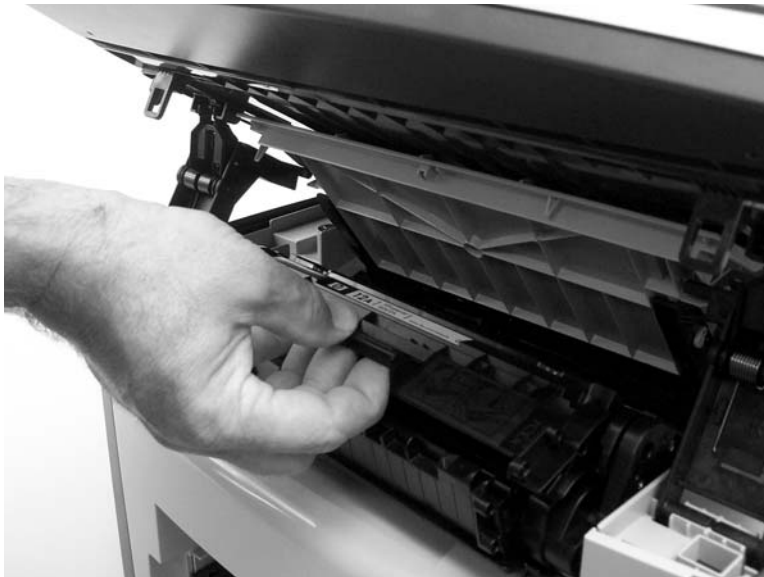
Figure 6-48 Removing the print cartridge (2 of 2)
