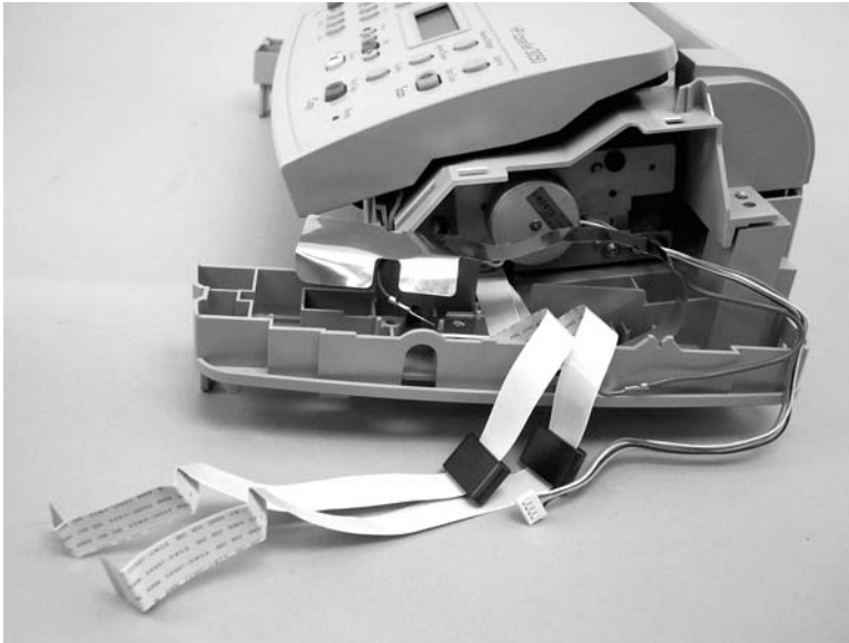
Figure 6-35 Removing the scanner assembly top cover (2 of 4)
