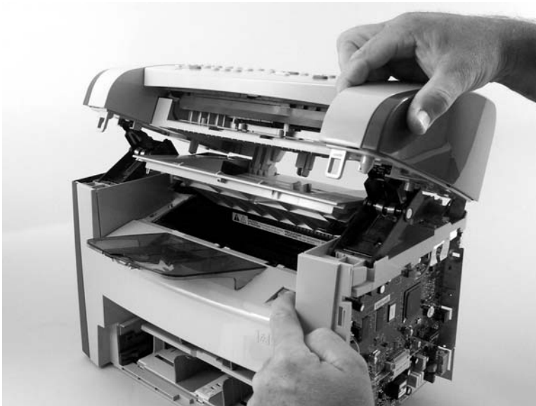
Figure 6-27 Removing the scanner assembly (8 of 14)
