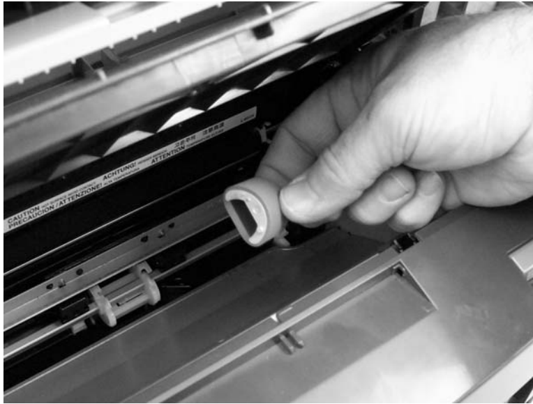
Figure 6-51 Removing the pickup roller (3 of 5)
