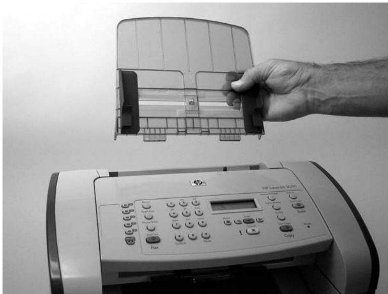
Figure 6-20 Removing the scanner assembly (1 of 14)
