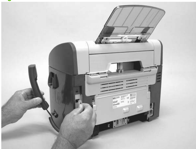
Figure 6-44 Remove the handset
