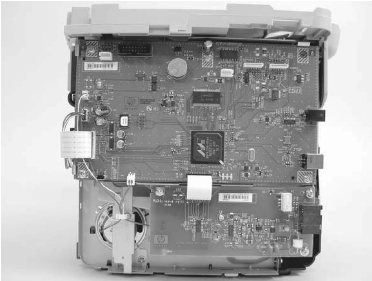
Figure 6-83 Removing the formatter (2 of 4)
