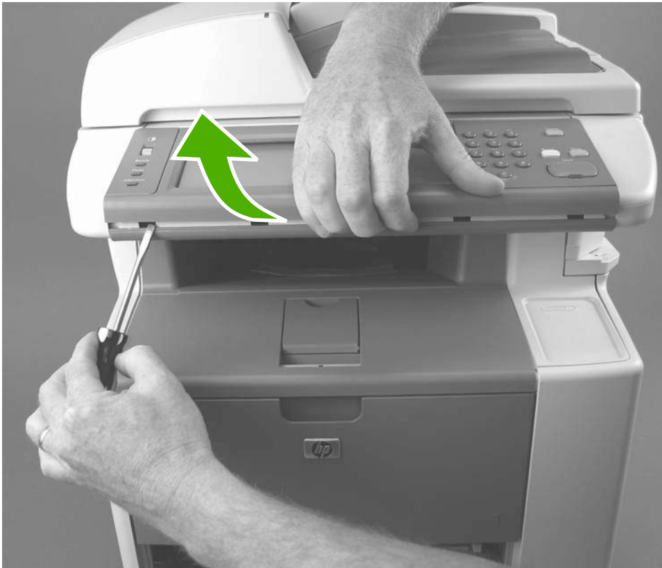
Figure 5-6 Removing the control panel (1 of 2)
