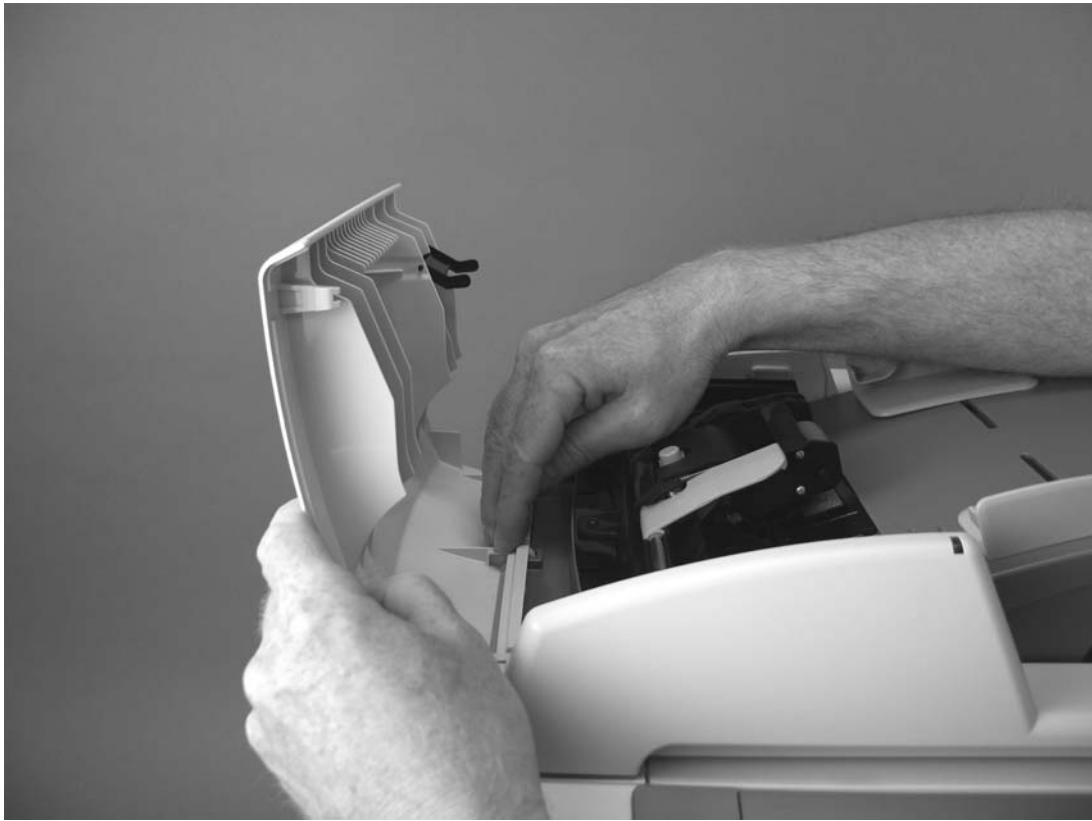
Figure 5-3 Reinstalling the ADF cover
