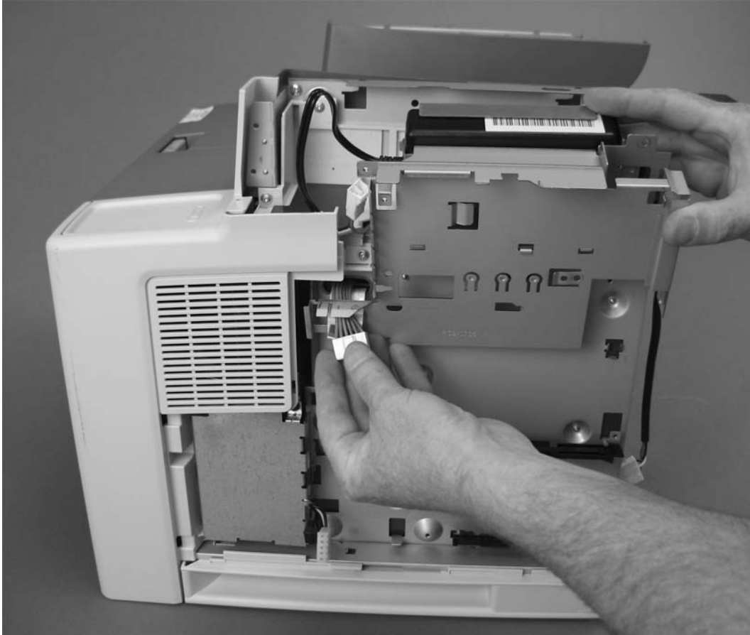
Figure 5-47 Removing the stapler power supply (4 of 5)
