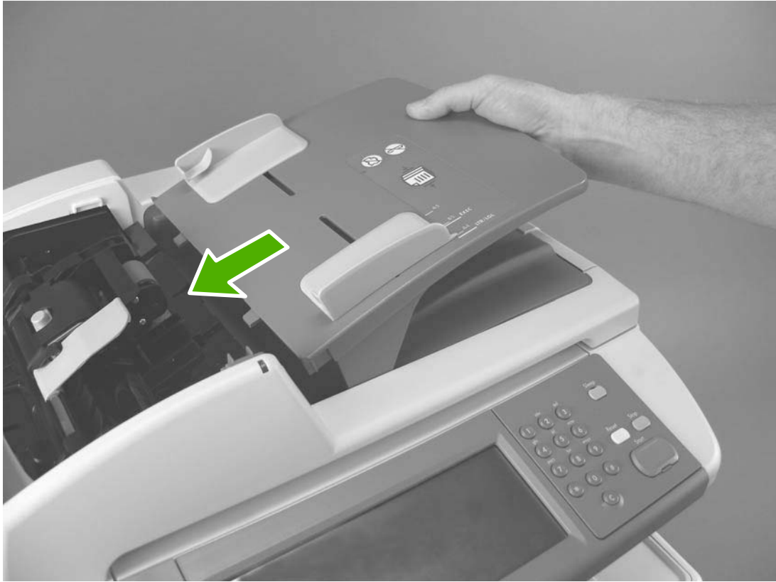
Figure 5-5 Reinstalling the ADF input tray
