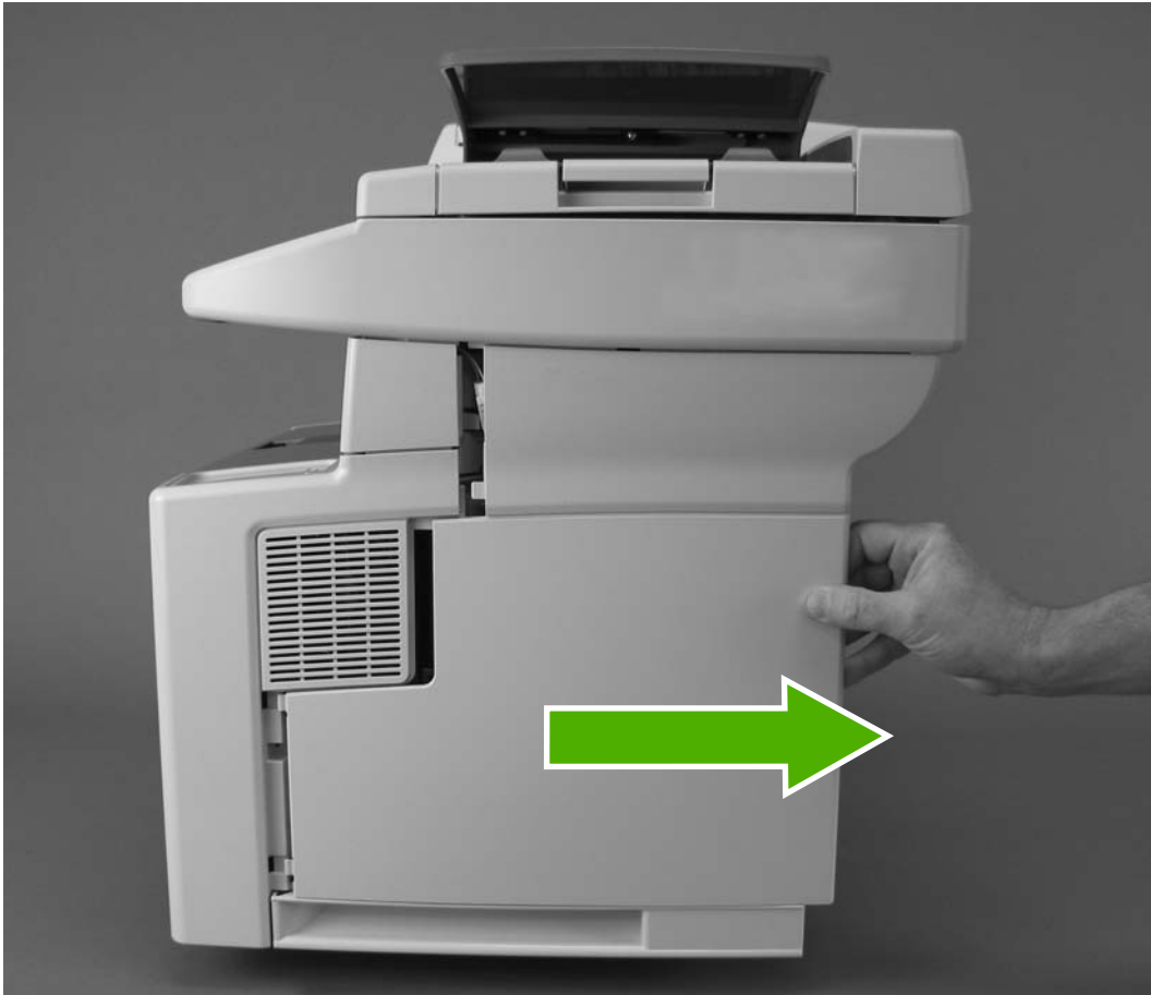
Figure 5-16 Removing the right-side cover
