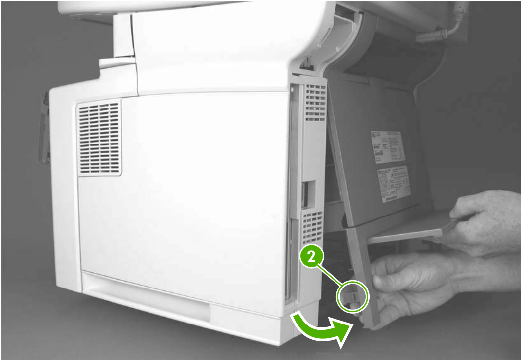
Figure 5-23 Removing the back cover (2 of 2)
