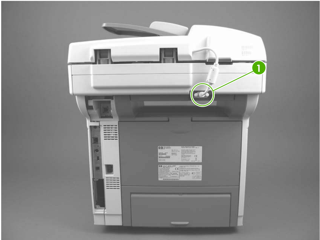
Figure 5-9 Removing the ADF (1 of 3)
