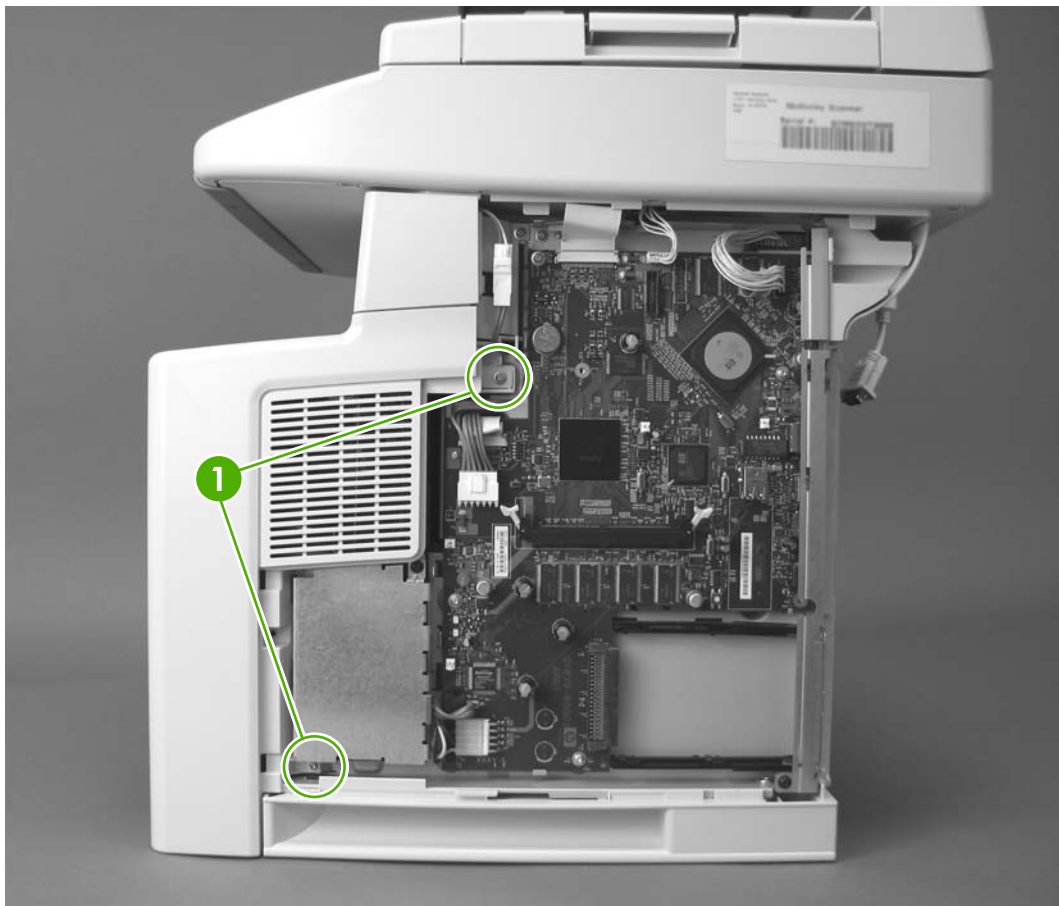
Figure 5-30 Removing the front, right cover (1 of 2)
