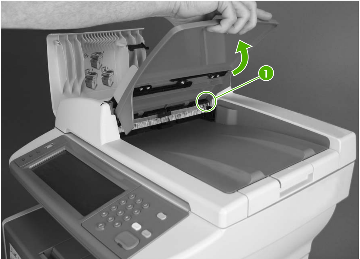
Figure 5-4 Removing the ADF input tray
