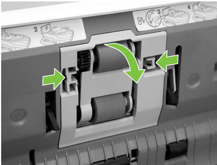
Figure 5-7 Remove the ADF separation pad and pickup and feed roller assemblies (4 of 5)
