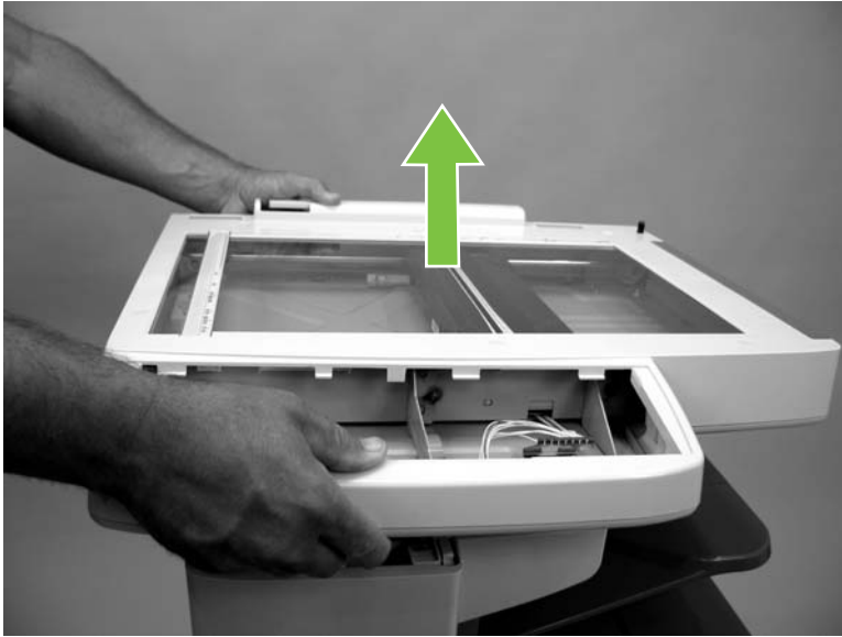
Figure 5-88 Remove the scanner (4 of 4)
