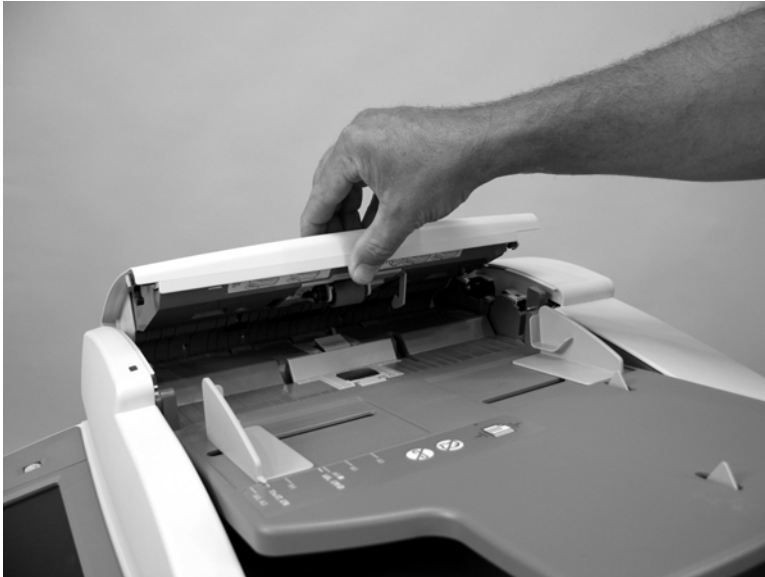
Figure 5-44 Remove the ADF separation floor assembly (1 of 4)
