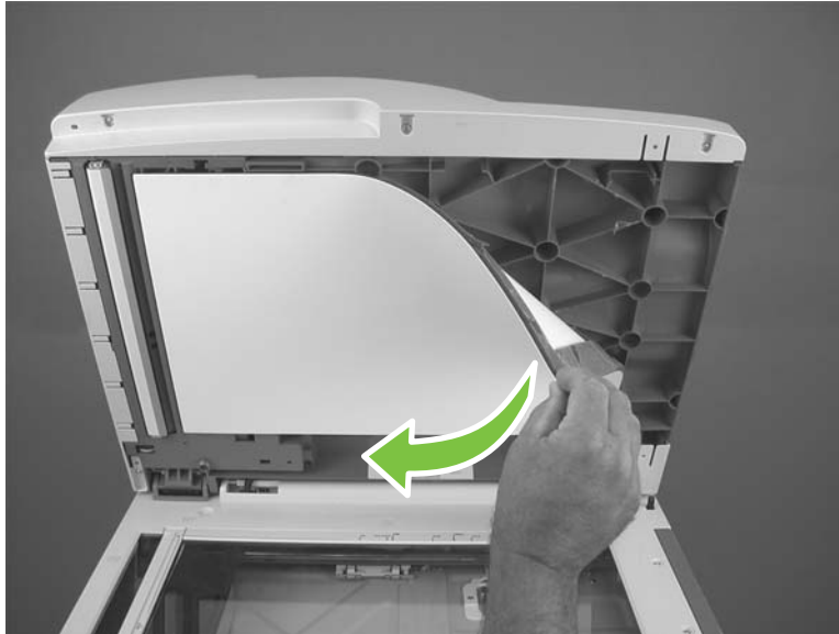
Figure 5-59 Remove the ADF white backing (1 of 4)
