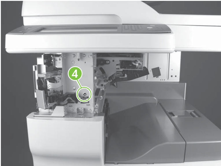
Figure 5-158 Remove the stapler alignment and jogger guide assembly (3 of 6)
