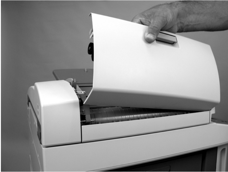
Figure 5-52 Remove the ADF jam cover (3 of 3)
