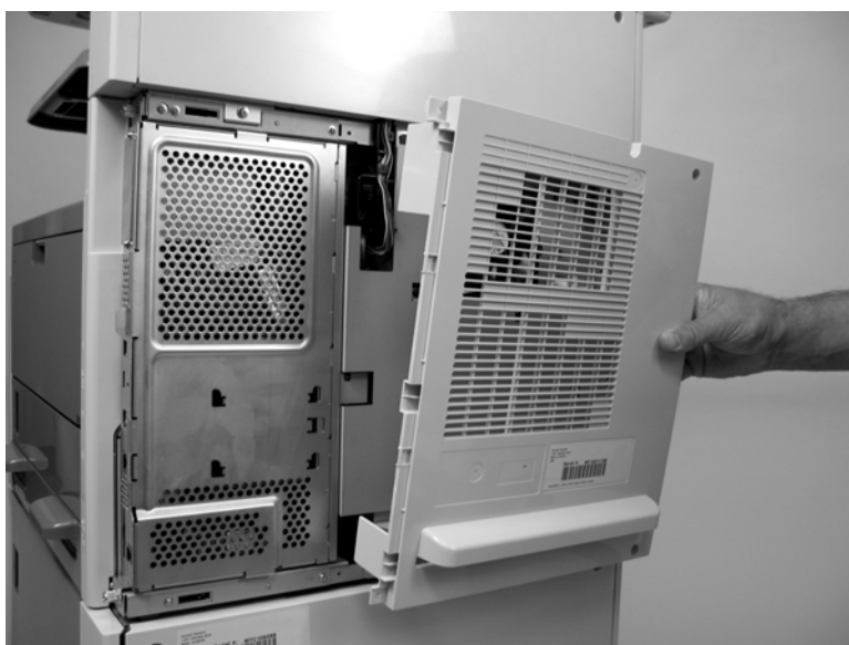
Figure 5-184 Remove the base unit rear cover (2 of 2)
