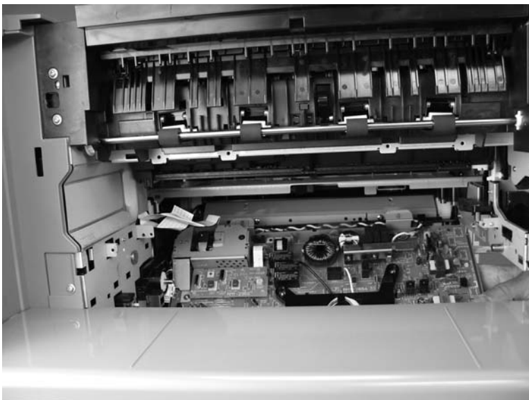
Figure 5-268 Reinstall the high-voltage power supply assembly (1 of 3)
