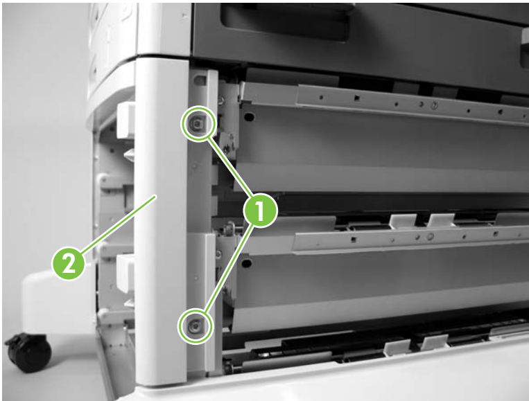
Figure 5-296 Remove the HCI front door (single tray unit only) (1 of 2)
