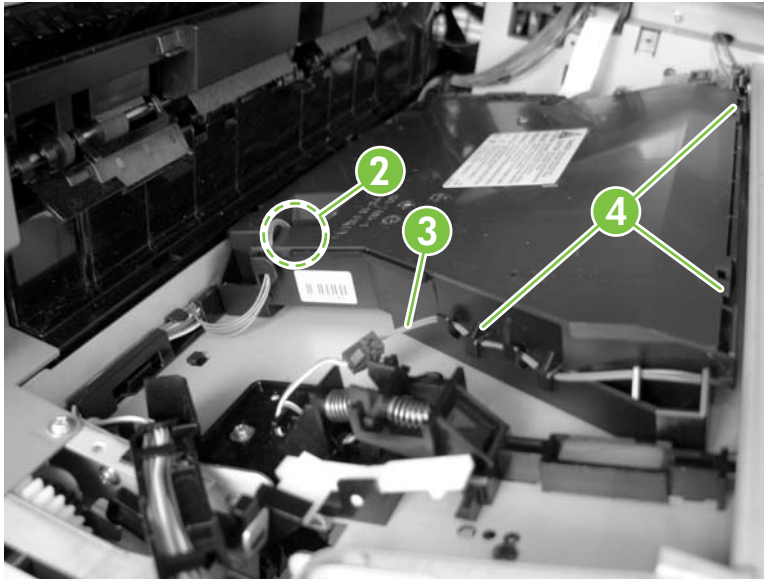
Figure 5-250 Remove the laser/scanner (2 of 3)
