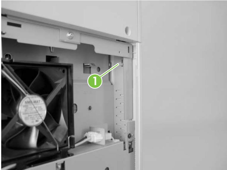
Figure 5-206 Remove the base unit left rear cover (1 of 2)
