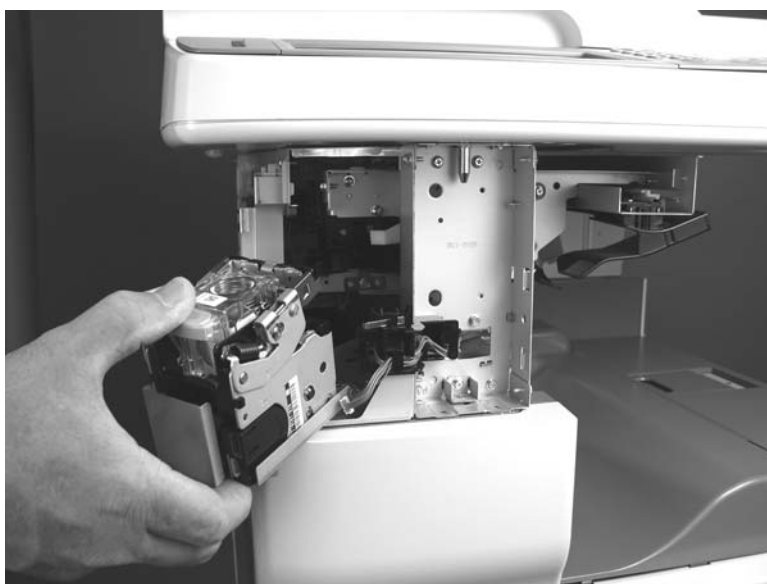
Figure 5-151 Remove the stapler unit (2 of 2)
