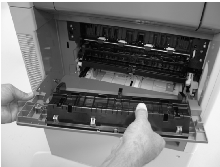
Figure 5-26 Remove the fuser (4 of 6)
