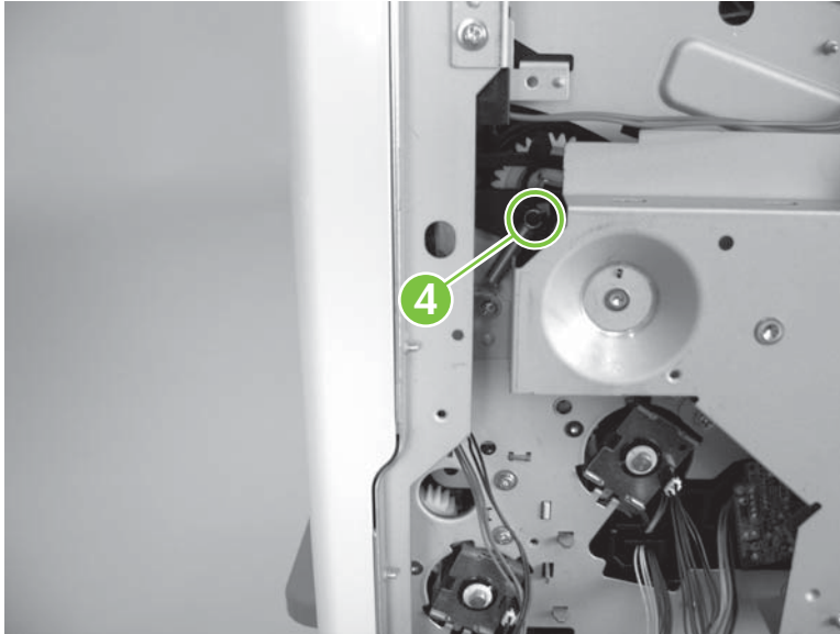
Figure 5-285 Remove the main motor (4 of 7)
