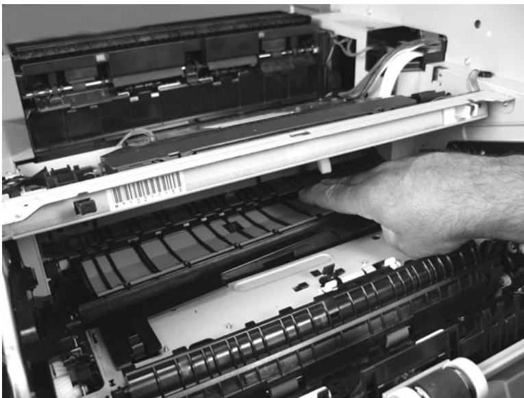
Figure 5-244 Reinstall the paper feed assembly (6 of 8)
