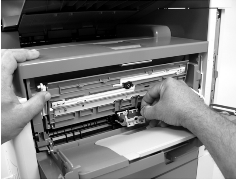
Figure 5-15 Remove the Tray 1 separation pad assembly (3 of 3)
