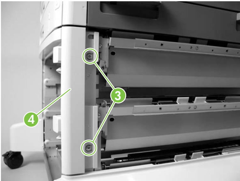
Figure 5-308 Remove the HCI paper pickup assembly (2 of 6)
