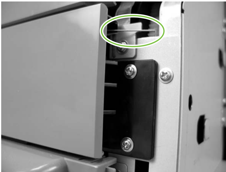
Figure 5-200 Install the base unit right door
