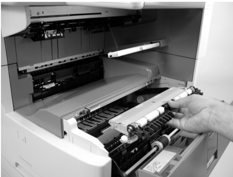
Figure 5-230 Remove the registration assembly (4 of 5)
