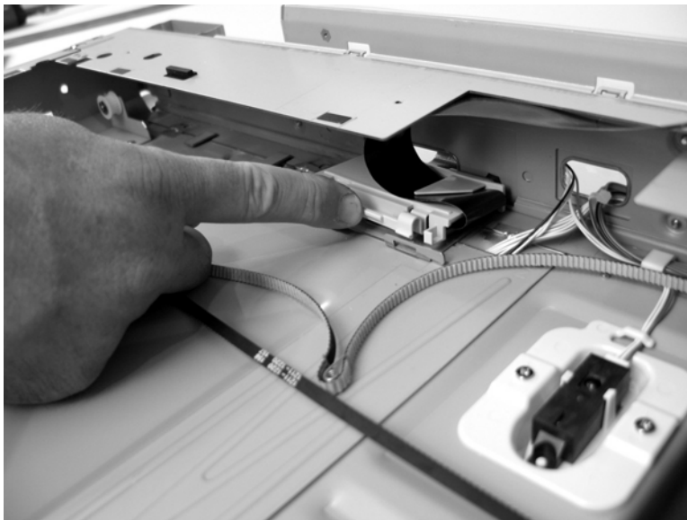
Figure 5-107 Remove the scanner optic assembly (12 of 13)
