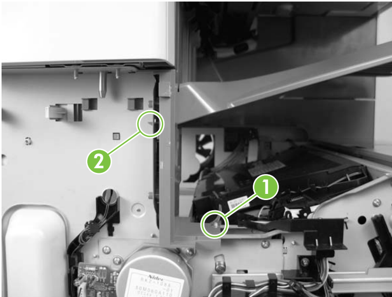
Figure 5-192 Remove the base unit face-down side cover (1 of 2)
