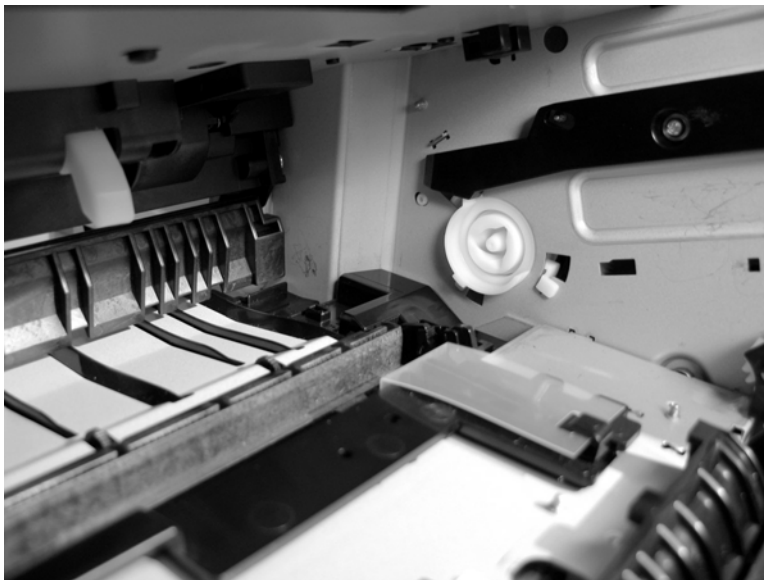
Figure 5-246 Reinstall the paper feed assembly (8 of 8)
