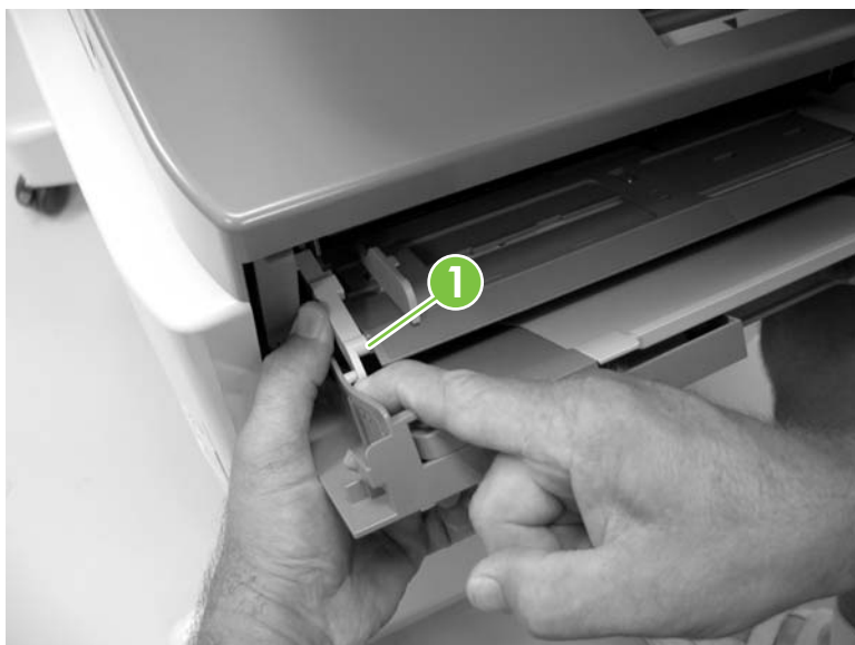
Figure 5-13 Remove the Tray 1 separation pad assembly (1 of 3; front retainer shown)
