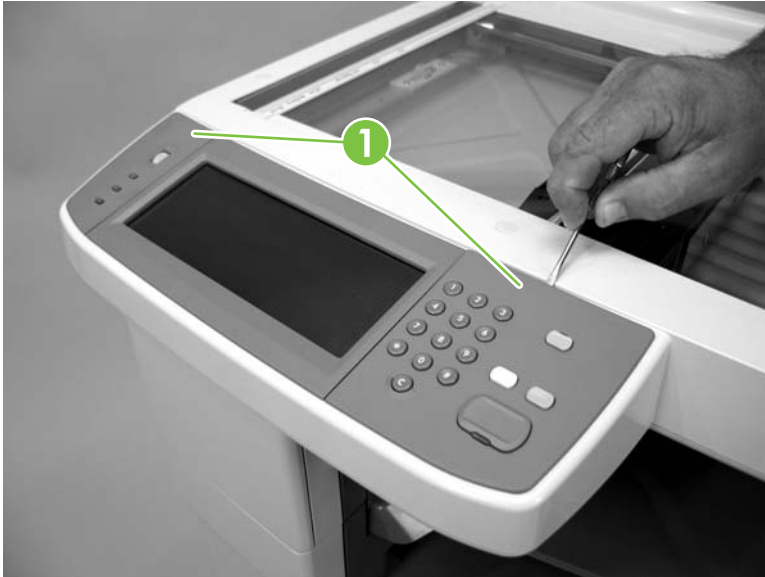
Figure 5-78 Remove the control panel (1 of 3)
