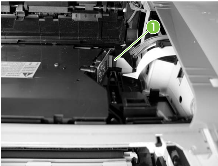
Figure 5-249 Remove the laser/scanner (1 of 3)
