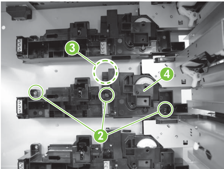
Figure 5-319 Remove the HCI lifter driver assembly (2 of 2)
