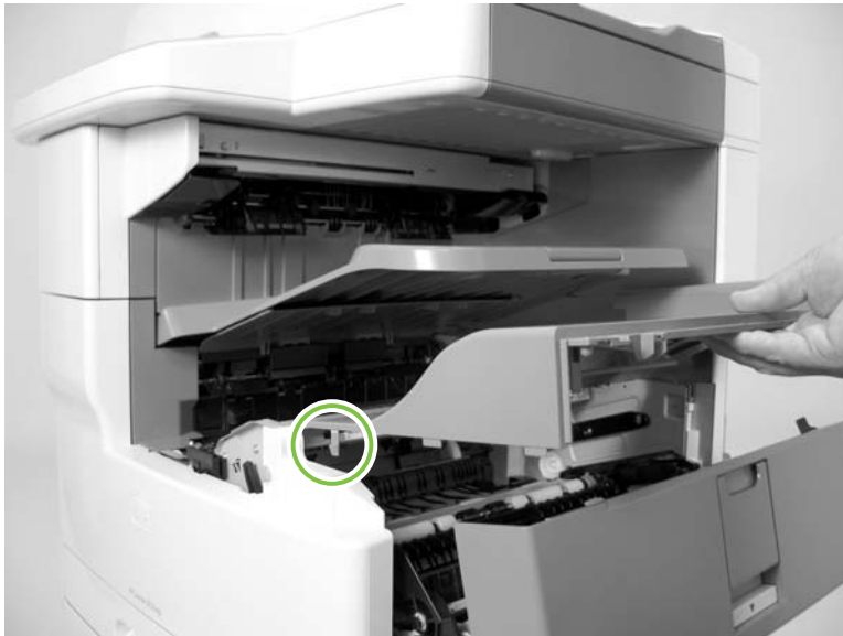
Figure 5-177 Remove the base unit face-down cover (2 of 2)
