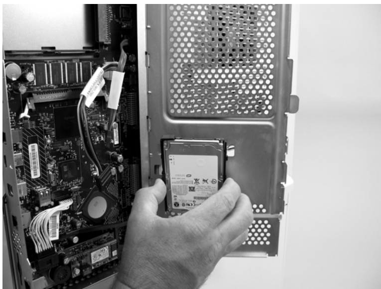
Figure 5-35 Remove the hard drive (2 of 2)
