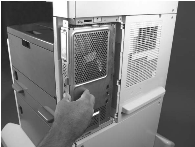
Figure 5-33 Reinstall the formatter cage
