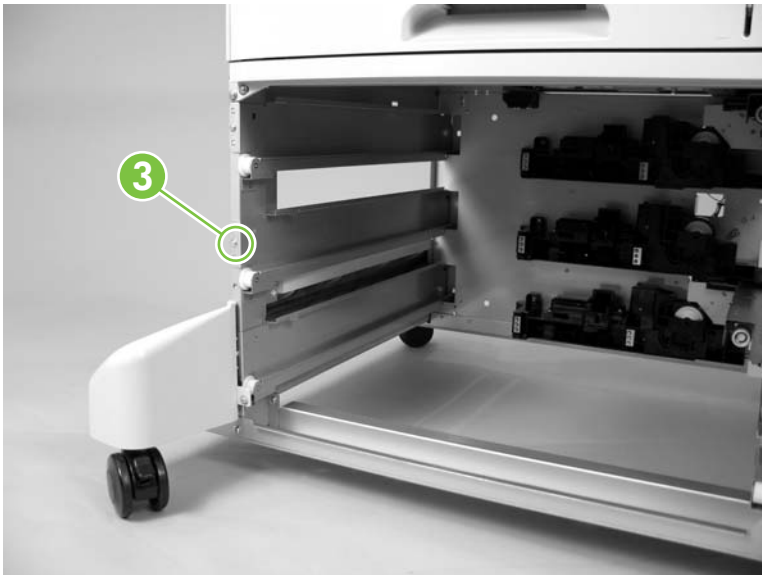
Figure 5-316 Remove the HCI left side tray rail(s) (2 of 3)
