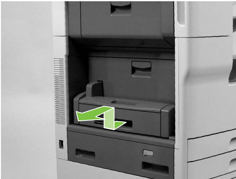
Figure 5-29 Remove the duplexer
