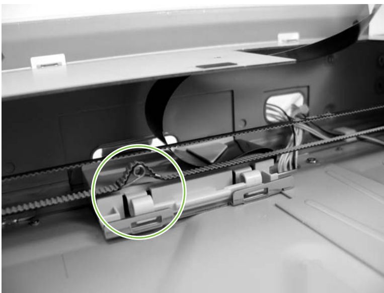
Figure 5-105 Remove the scanner optic assembly (10 of 13)
