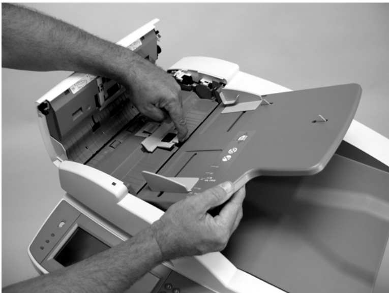
Figure 5-5 Remove the ADF separation pad and pickup and feed roller assemblies (2 of 5)
