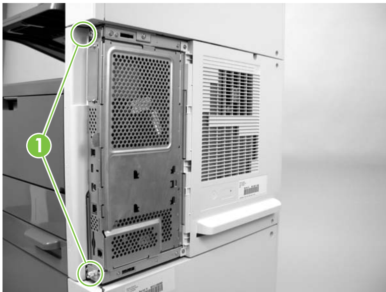
Figure 5-31 Remove the formatter cover and cage (2 of 3)
