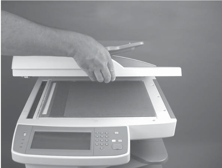
Figure 5-61 Remove the ADF white backing (3 of 4)
