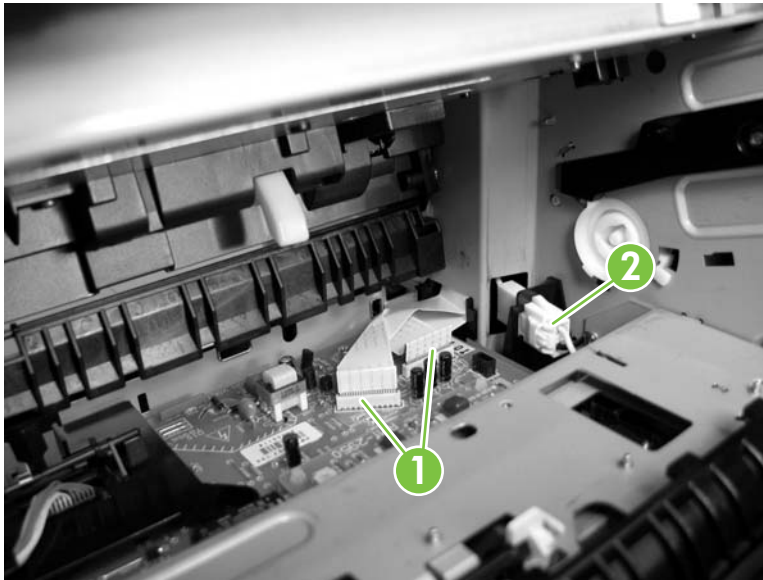
Figure 5-259 Remove the high-voltage power supply assembly (1 of 9)
