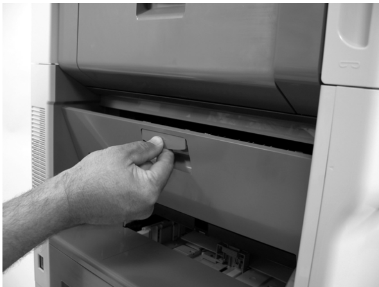
Figure 5-24 Remove the fuser (2 of 6)
