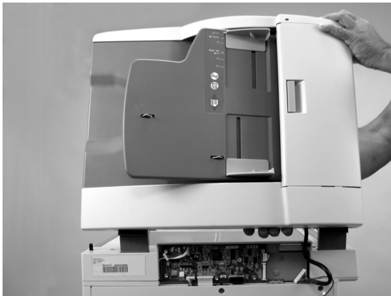
Figure 5-41 Remove the ADF (4 of 4)
