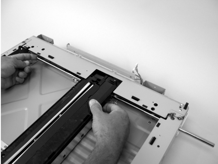
Figure 5-100 Remove the scanner optic assembly (5 of 13)
