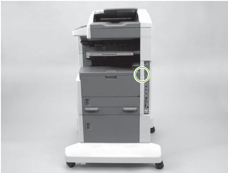
Figure 6-1 Engine test button location
