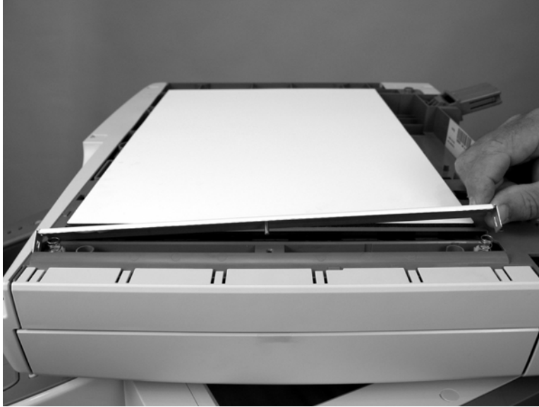
Figure 5-56 Remove the ADF float assembly (3 of 5)
