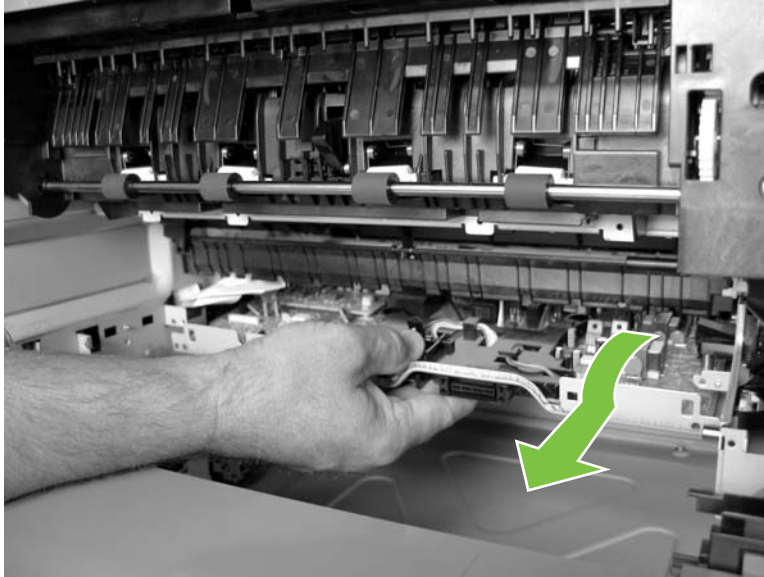
Figure 5-266 Remove the high-voltage power supply assembly (8 of 9)
