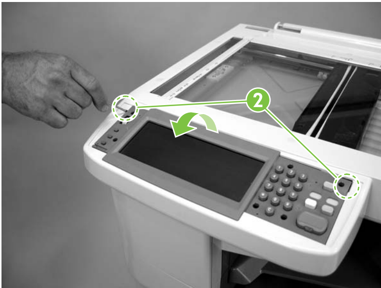
Figure 5-79 Remove the control panel (2 of 3)
