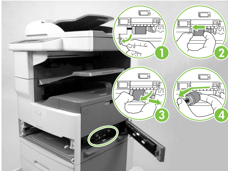
Figure 5-18 Remove the Tray 2 and Tray 3 pickup rollers (3 of 4)
