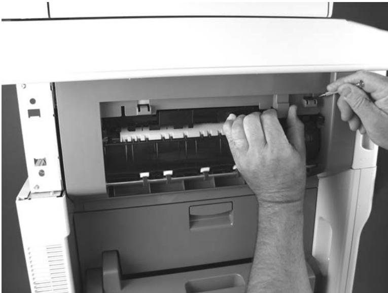
Figure 5-134 Remove the stapler left cover (1 of 3)
