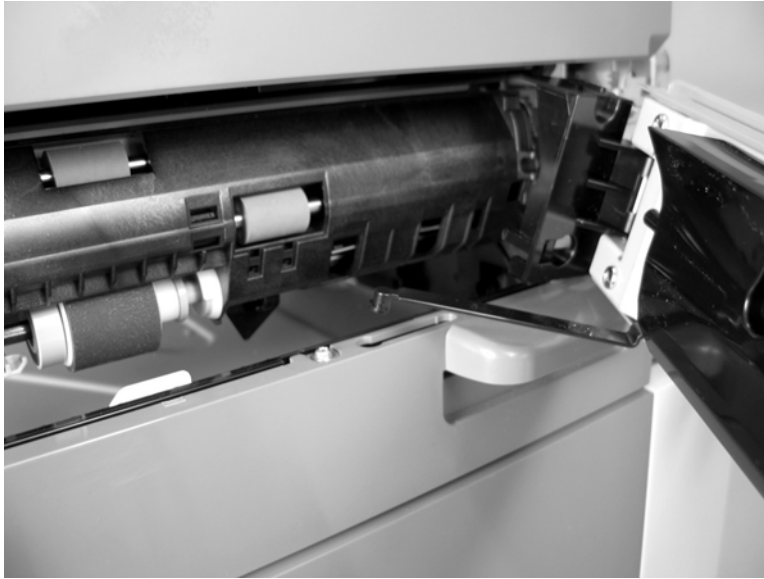
Figure 5-199 Remove the base unit right door (2 of 2)
