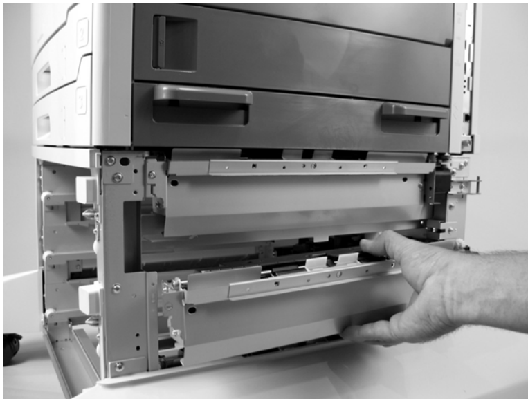
Figure 5-310 Remove the HCI paper pickup assembly (4 of 6; middle paper pickup assembly shown)
