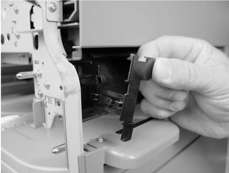
Figure 5-294 Remove the lower cassette pickup assembly (4 of 5)
