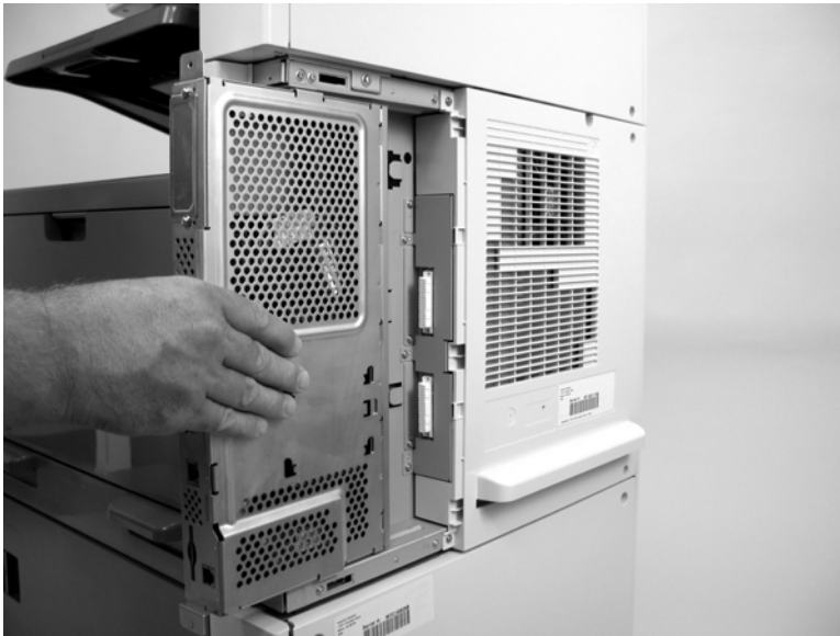
Figure 5-32 Remove the formatter cover and cage (3 of 3)
